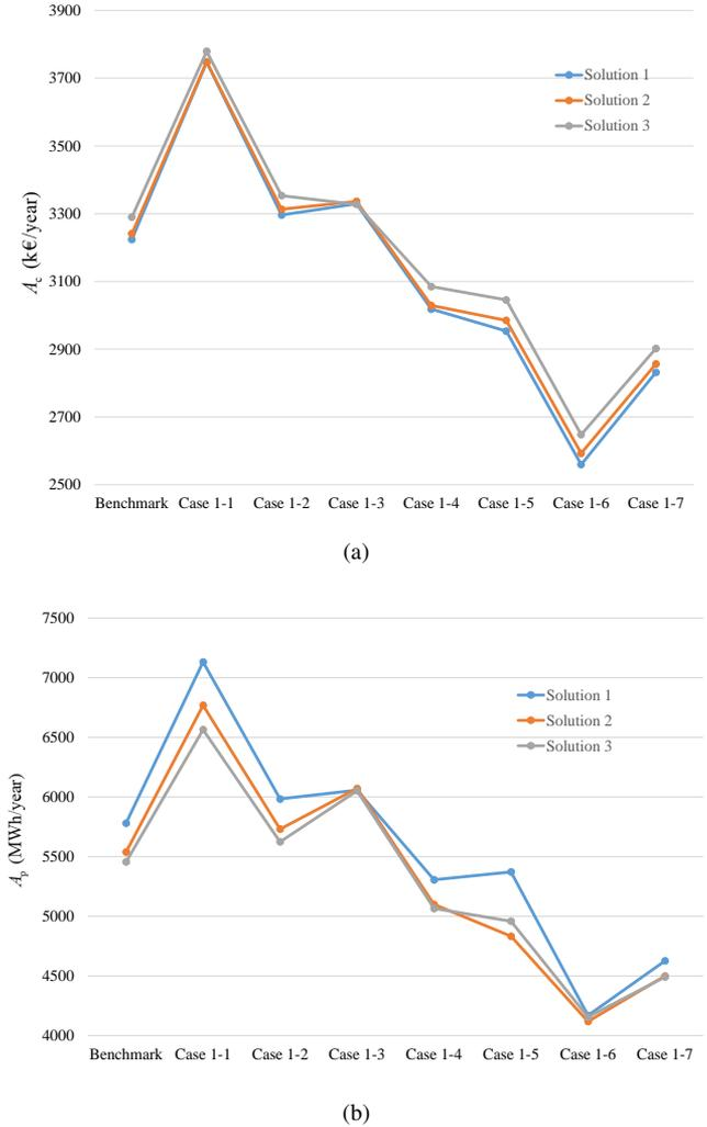
Figure 4.7: Comparison of Cases 1-1 to 1-7: (a) Maintenance cost (b) Production loss
