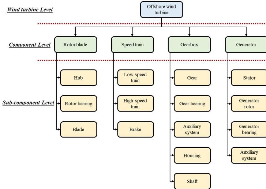
Figure 5.1: Hierarchical levels of offshore wind turbine
