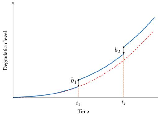
Figure 3.1: Abrupt increases of degradation caused by influential impact
