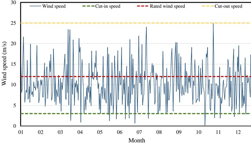
Figure 4.5: Wind speed and turbine design parameter
