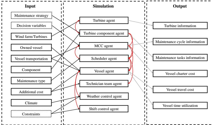
Figure 6.1: The framework for vessel fleet management
