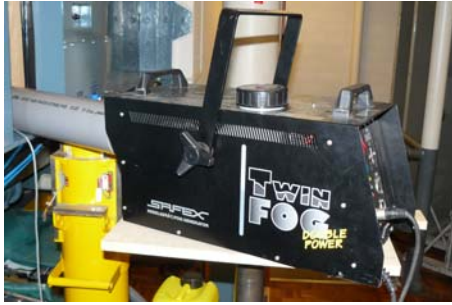
Figure 10.18: Smoke generator producing droplets of 1\ \mu m
