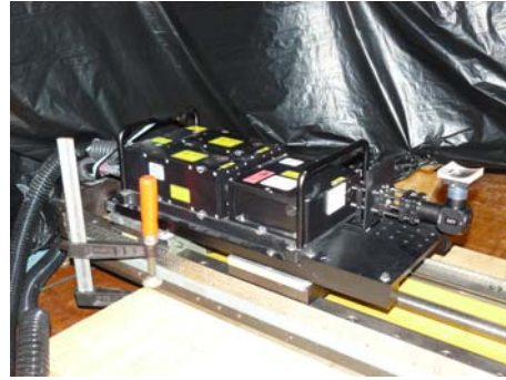
Figure 10.19: Laser setup underneath the windtunnel
