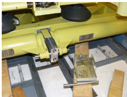
Figure 10.7: Model support structure with aluminum \alpha -adjustment block
