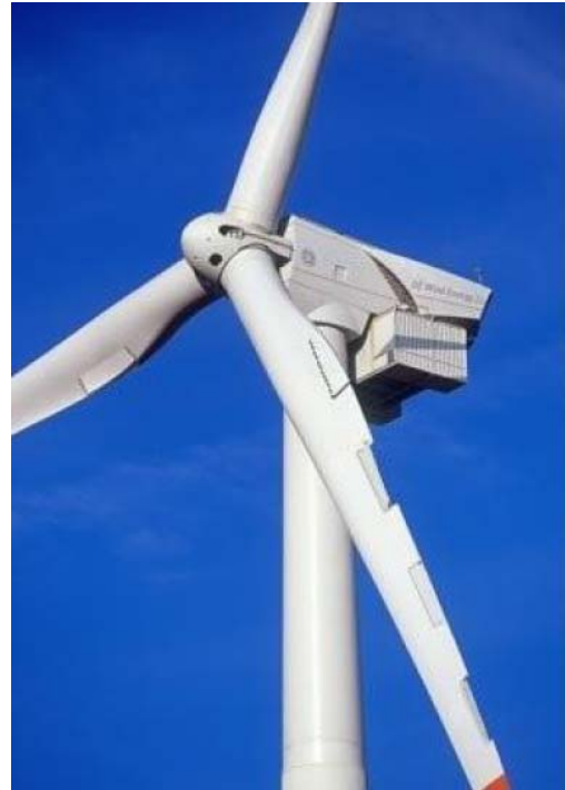
Figure 2.2: The Smart Rotor Blade applied on a wind turbine, showing a distribution of trailing edge flaps over the span of the rotor
