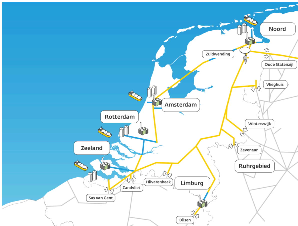
Figure 4.2: Hydrogen grid of the Netherlands in 2030 according to Gasunie
