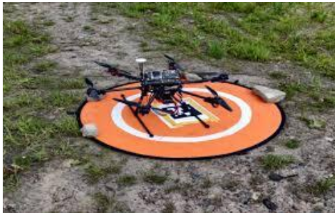
Figure 2.2: Usage of April Tag for UAV Landing [32]
