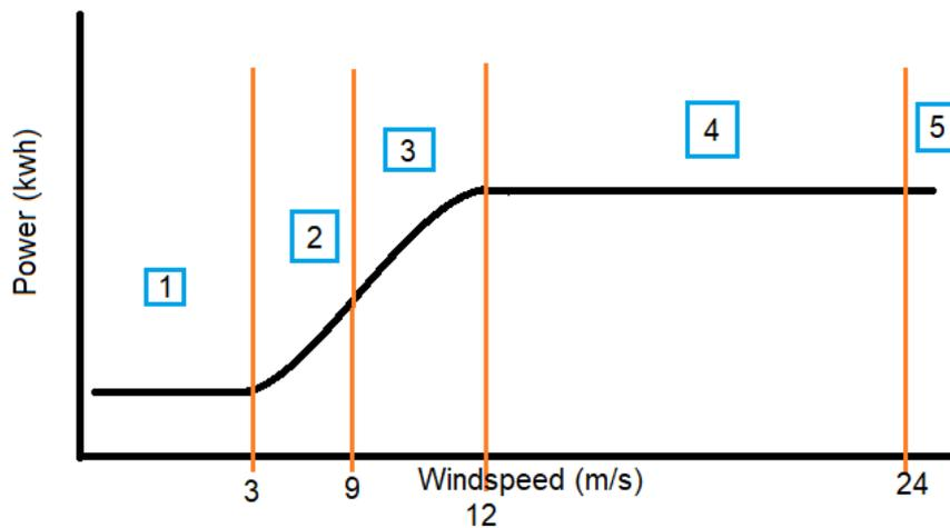
Figure 3.2 Operational regions of a wind turbine
