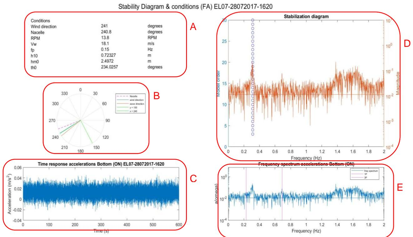
Figure 5.1 Stability diagram and conditions EL07 datasample 28072017 16:20h in the FA direction
