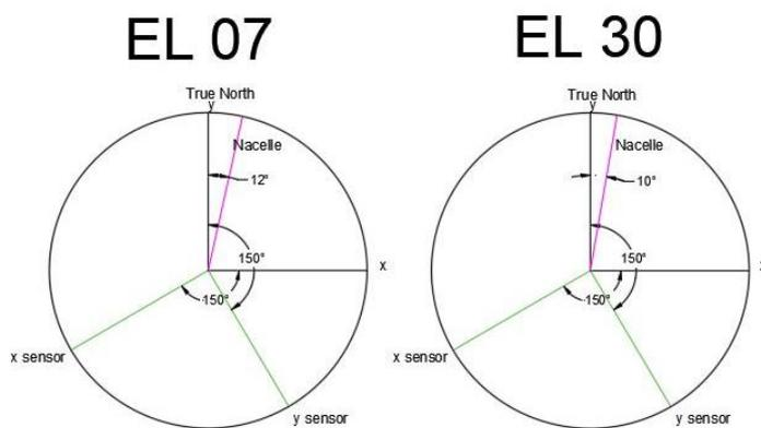
Figure 3.9 Orientation Nacelle and sensors with respect to the true North
