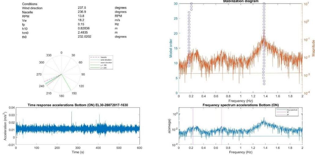
Figure 5.14 Stability diagram and conditions data sample for EL30 28072017 16:30h in the FA direction.
