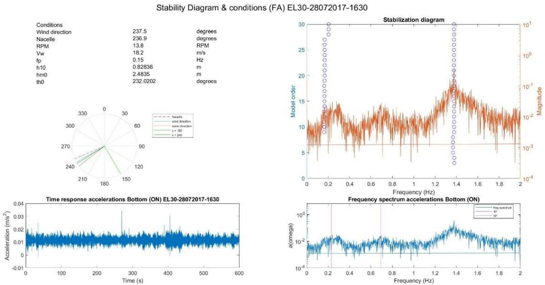
Figure 5.16 Stability diagram and conditions data sample for EL30 28072017 16:30h in the FA direction
