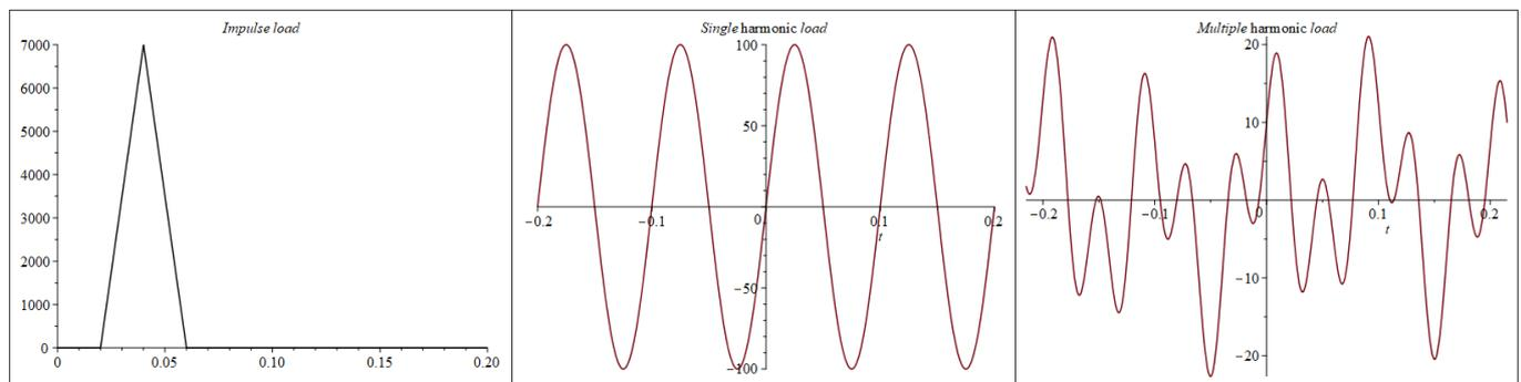
Figure 2.2 Load cases beam model
