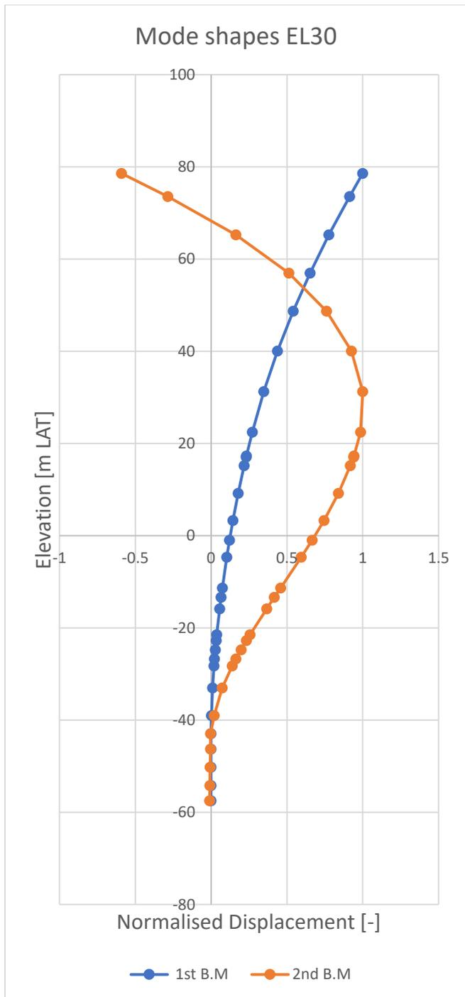
Figure 3.4 Design Mode shapes turbine EL30
