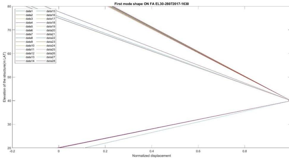
Figure 5.7 ‘First’ Mode shapes (model order 3 to 30) data sample EL30 28072017 16:30h
