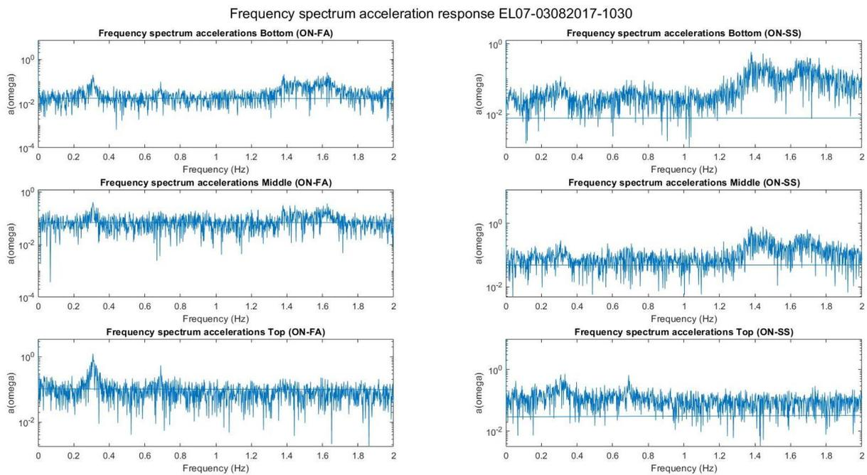
Figure 3.11 Frequency spectra in the FA/SS for EL07
