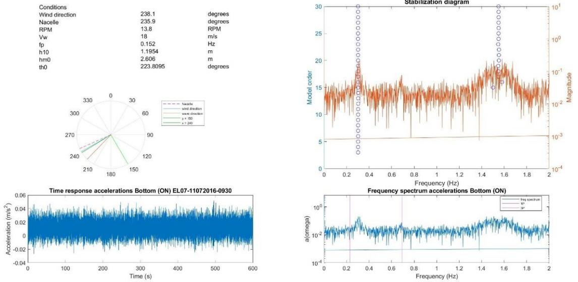
Figure 5.15 Stability diagram and conditions data sample for EL07 11012017 9:30h
