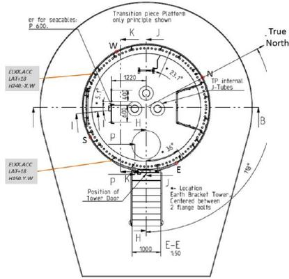
Figure 3.8 Orientation of the sensors
