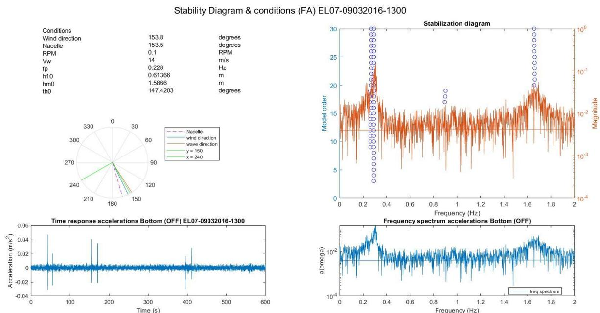
Figure 5.17 Stability diagram and conditions data sample for EL07 09032016 13:00h
