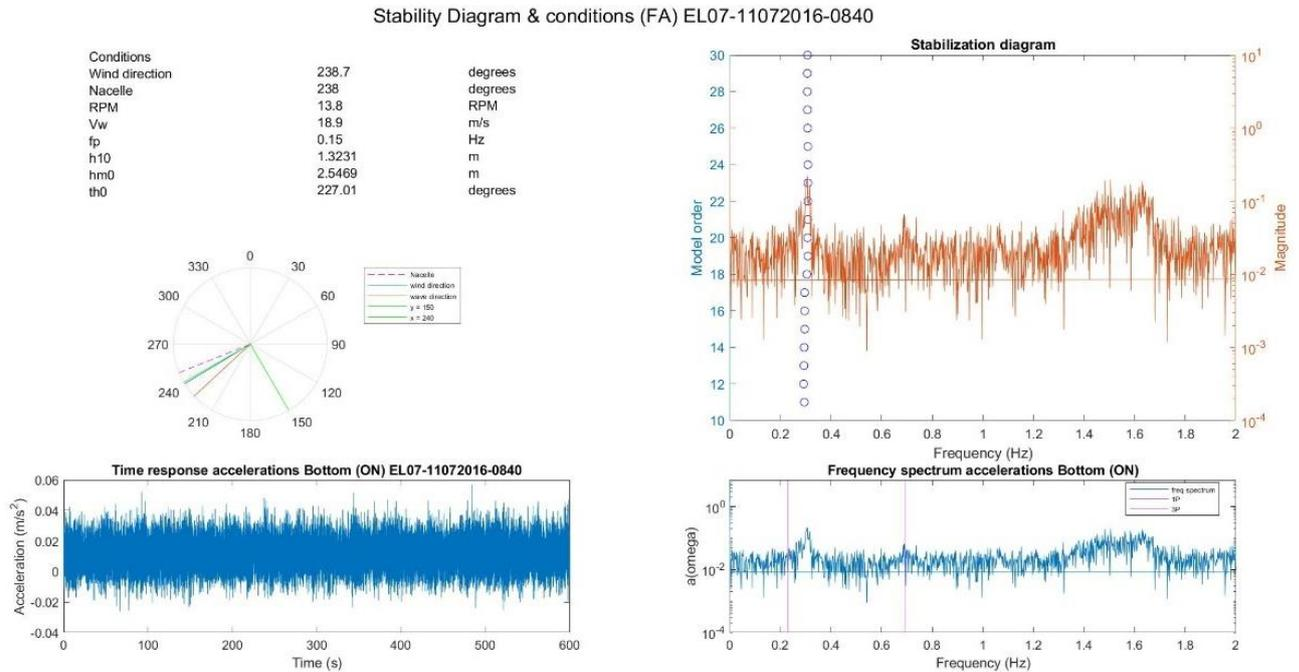
Figure 5.9 Stability diagram and conditions data sample EL07 for 11072016 8:40h in the FA direction
