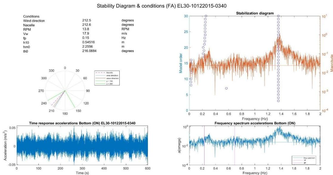
Figure 5.6 Stability diagram and conditions data sample EL30 for 28072017 16:30h in the FA direction
