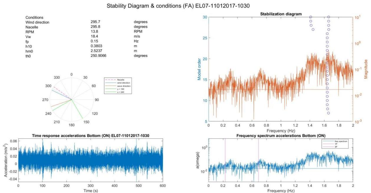
Figure 5.4 Stability diagrams and conditions data sample EL07 for 11012017 at 10:30h in the FA direction
