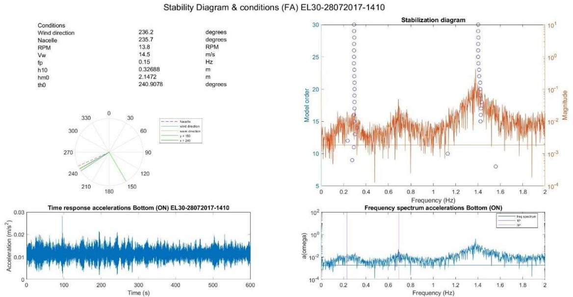
Figure 5.12 Stability diagram and conditions data sample for EL30 28072017 14:10h in the FA direction
