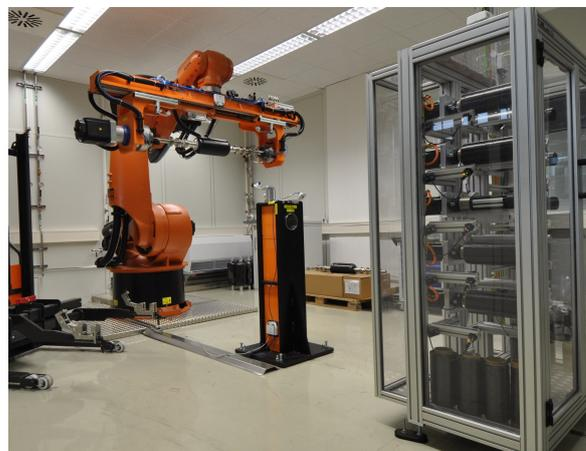
Figure 3.1: Robot-assisted filament winding system
