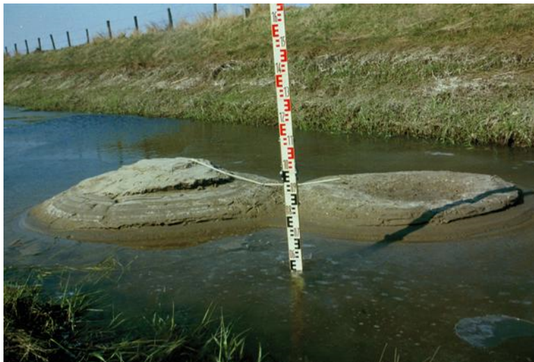
Figure 1.2: Sand boils. Source:[Rijkswaterstaat,2014].
