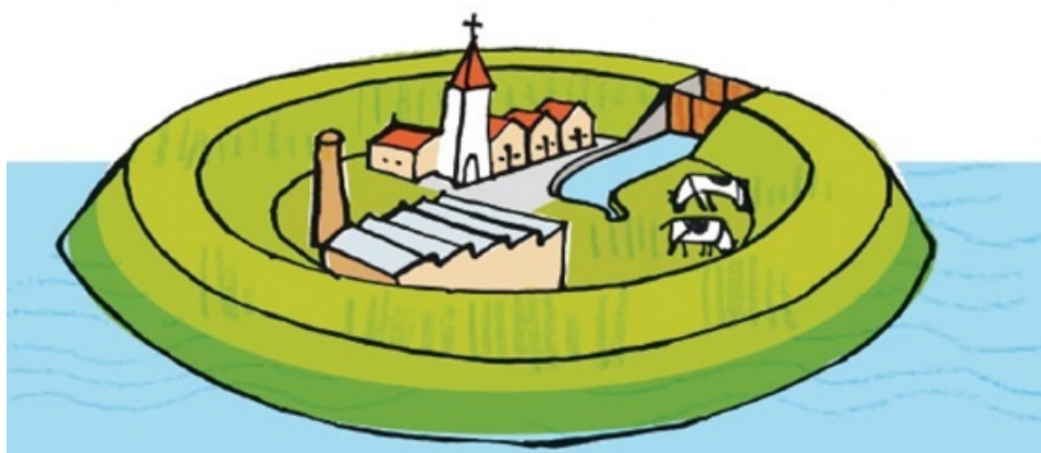
Figure 2.3: Dike ring schematization. Source: [Rijkswaterstaat,2012].
