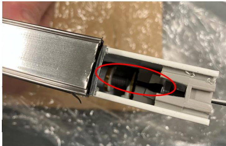
Figure 16: Temperature sensor embedded in the IGU spacer. Its recorded data is an approximation to the operational temperature of the bPV cells.
