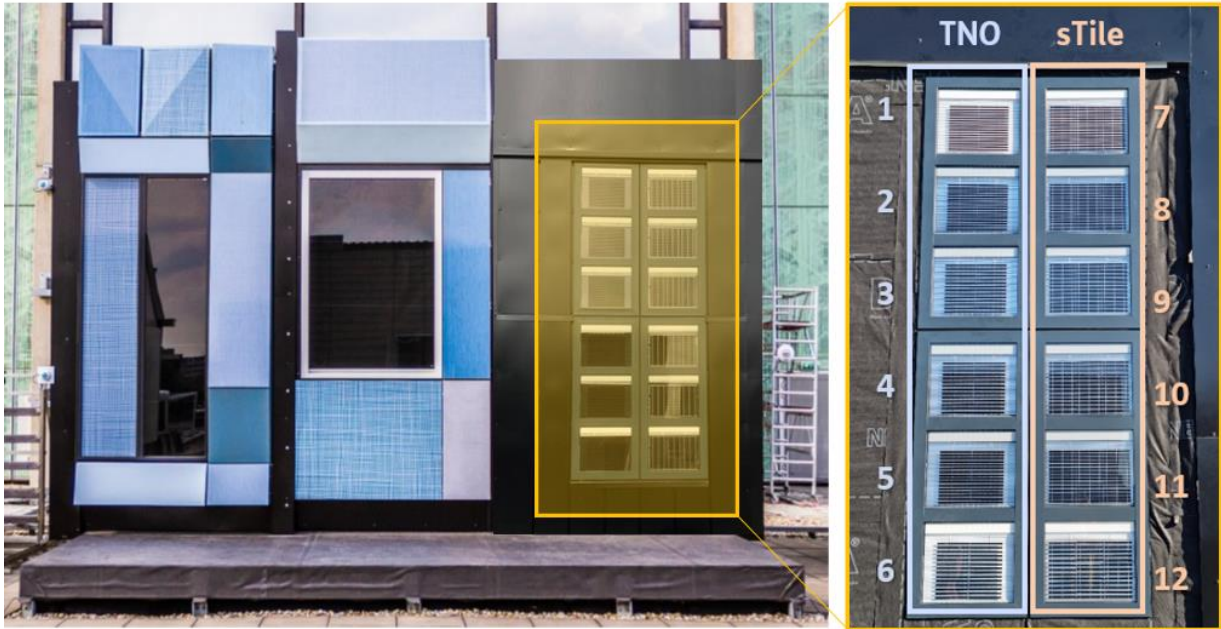
Figure 7: (left) the dummy building at SolarBEAT , in which the 12 bPV window demonstrators have been installed (at the right side). (Right): numbering of the bPV window demonstrators for identification purposes. Source: TNO internal.
