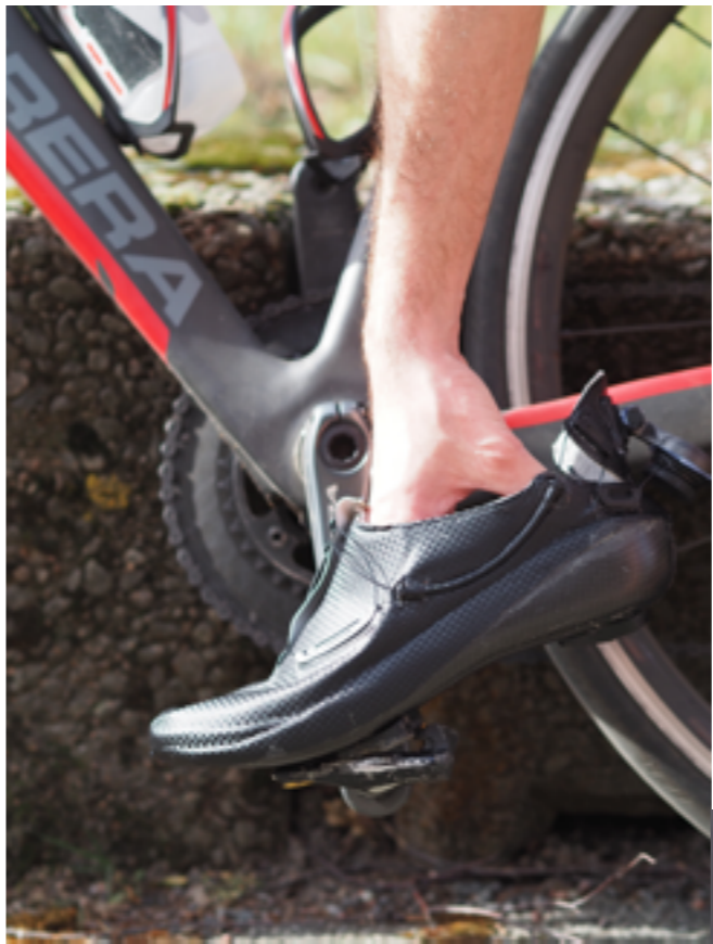
Step 1: Press the shoe on the pedal
