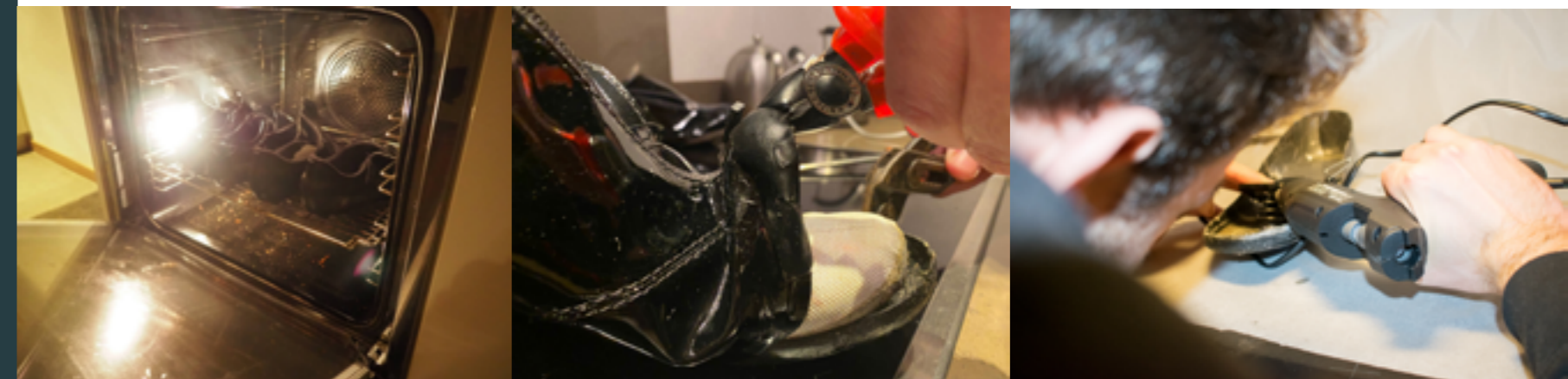
Image 48, 49 and 50: The process of heating the glue to take the padding away from the carbon sole. Afterwards a gluegun was used to re-apply the modified components.
