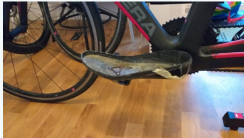
Image 51 to 53: Custom designed 3D-printed pins could hold the shoe horizontal by leaning on the frame. They were glued to the carbon sole for extra strength.
