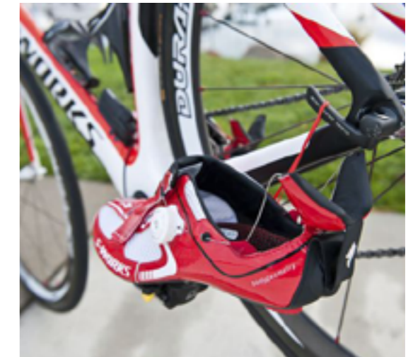
Image 4: Elastic bands to keep the shoe horizontal
