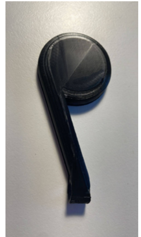
Image 65: Handle design based on company knowledge that it would be nice to have a dial winding button on it
