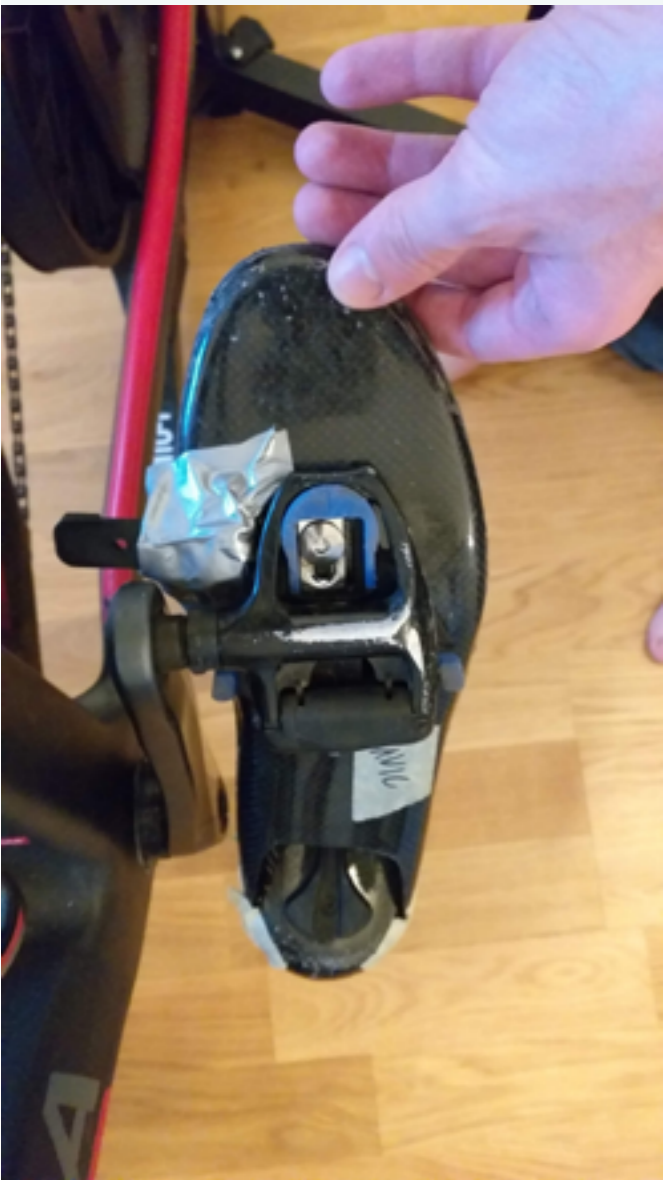
Image 51 to 53: Custom designed 3D-printed pins could hold the shoe horizontal by leaning on the frame. They were glued to the carbon sole for extra strength.
