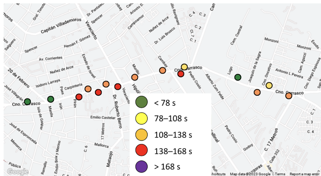
Figure 6. Line 109: mean delays on Camino Carrasco.
