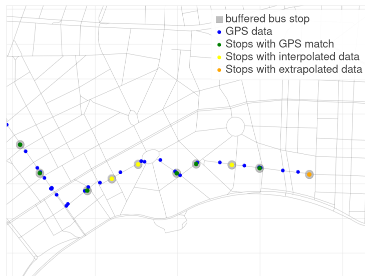
Figure 9. Assignment of travel times to stops on the final stretch of line 2 from Hospital Saint Bois to Playa Malvín.
