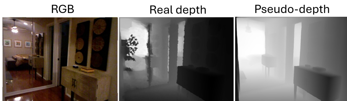
Figure 2.1: An RGB, real depth, and pseudo-depth image from the NYUDepthV2 [24] dataset. Real depth is more noisy, but has a more true-to-life value distribution. Semantic differences on the reflective surfaces are also visible; neither depth image is clearly superior.
