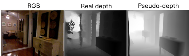
Figure 3. Image 1015 from NYUdepthv2 [15]: RGB, real depth, pseudo-depth. Real depth is noisier but displays absolute distance unlike pseudo-depth, which consequently has a different value distribution. Semantic differences also exist – the mirror is seen as noise in real depth, whereas pseudo-depth suggests the room extends into the mirror. Neither depth image is obviously strictly better.
