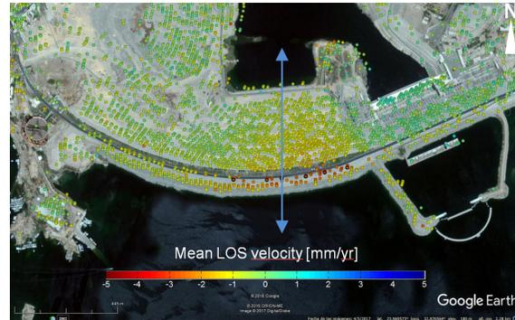
Figure 3. Mean LOS velocity derived from Envisat ASAR data.
