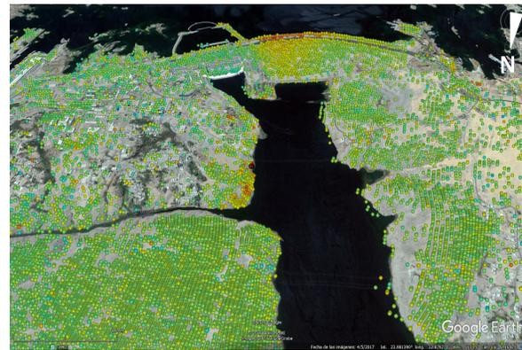
Figure 4. Location of a possible landslide 1 km north of the dam (red pixels in the center of the picture).
