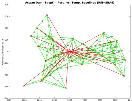
Figure 2. Perpendicular vs. temporal baselines distribution. Red and green connections correspond to PS and SB networks respectively.
