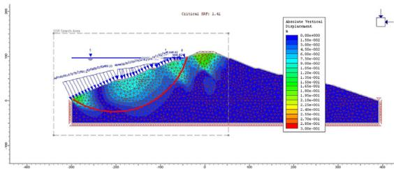
Figure 6. The deformed mesh from the FEM analysis.
