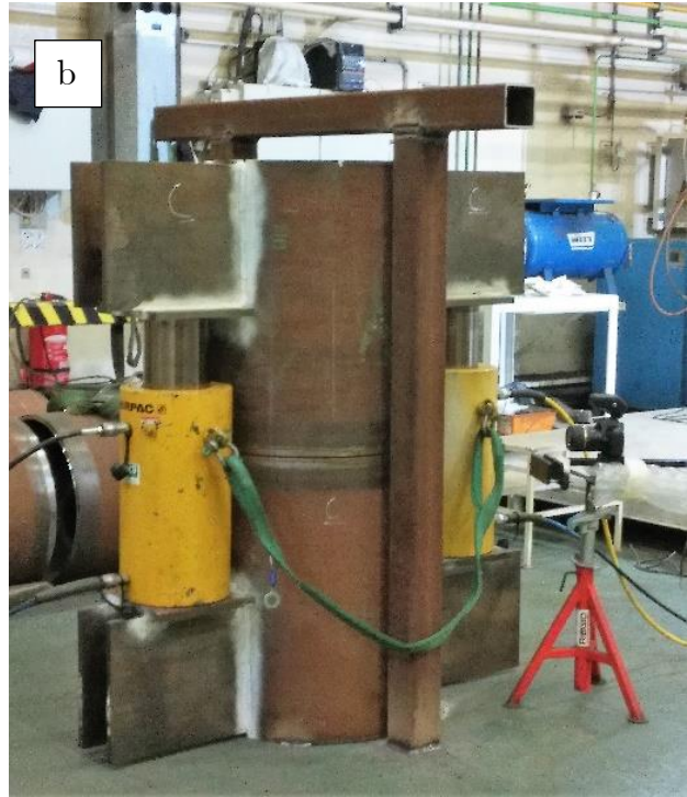
Figure 2.4a High Tonnage Cylinder, Enerpac model CLR25013, used for coupons overstressing (Enerpac, 2018); b) Test coupon C, just before the overstressing load application.
