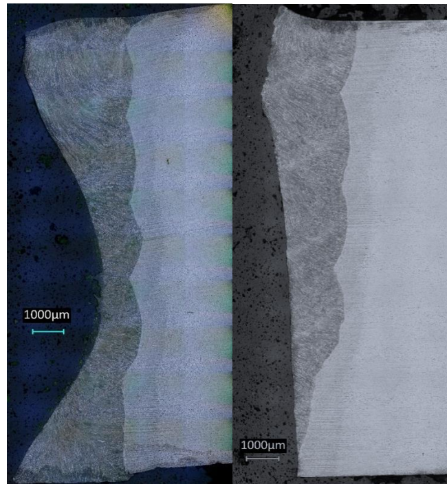
Figure 4.29 Specimen C-100, macrographs of the full weld, edge plane (left) and middle plane (right) views are presented.
