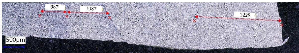
Figure 4.26 Hardness indents across the beadweld of specimen 0-2. Dimensions are given in μm.
