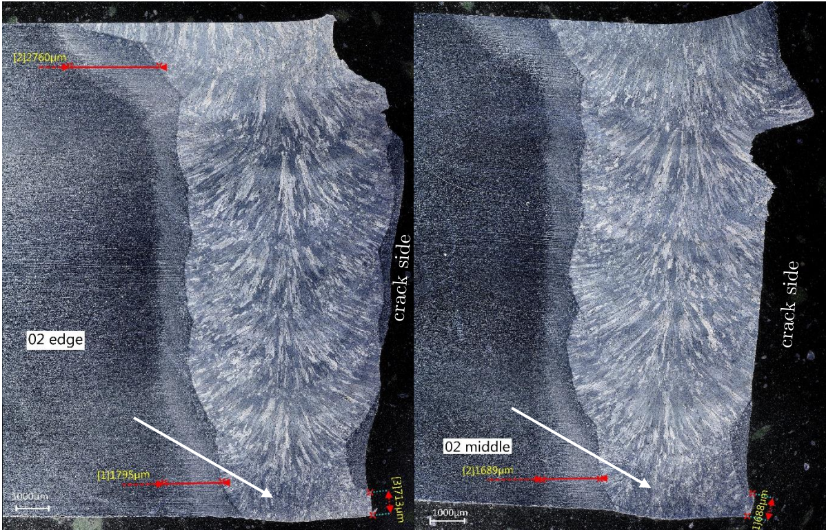
Figure 4.23 Specimen 0-2 edge plane and middle plane views of the full weld. Magnification x50. The beadweld is marked with the arrow.
