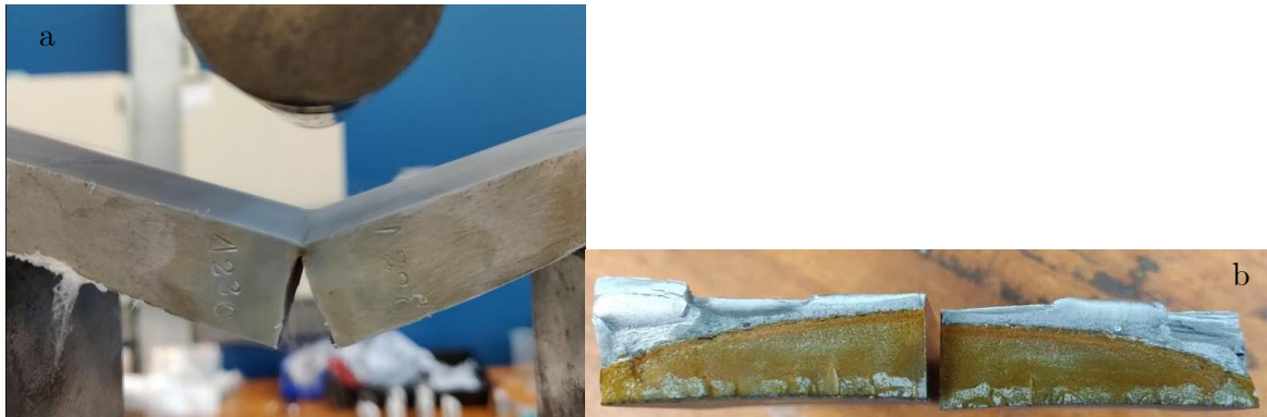
Figure 2.14 a) Specimen A-220, just before overload application, b) two halves of the specimen, with a clear distinction between FS (rusty area) and overload. Crack growth anisotropy clearly visible.
