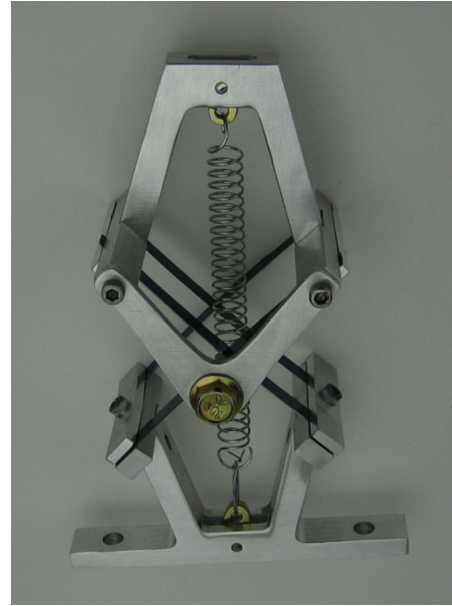
Fig. 8. Negative stiffness state & curved spring example. The helical spring is in a state of tension and counteracts the torque created by the leaf springs during rotation. Retrieved from [33].
