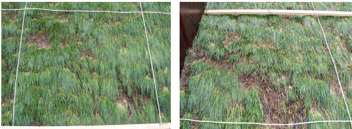
Figure 9-5: Detailed photographs of some bare spots after the '50' l/s/m test at the unreinforced test section
