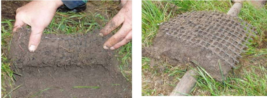
Figure 5-5: Details of dug up SGR samples of monitoring section 6 October 2006
