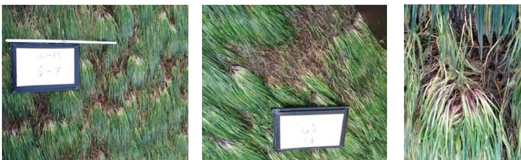
Figure 9-3: Detailed photographs of some bare spots after the 20 l/s/m test at the unreinforced test section
