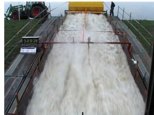
Figure 9-13: Situation during overtopping of 20 l/s/m. The biggest wave shown here had a volume of 3.5 m 3 per m width.
