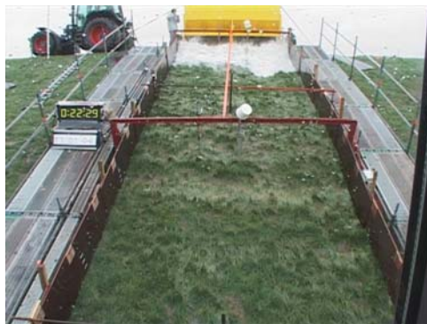
Figure 9-10: Situation during overtopping of 0,1 l/s/m. The biggest wave shown here had a volume of 0.7 m 3 per m width
