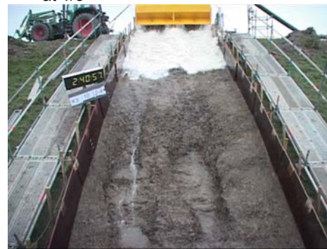
Figure 11-10: Situation during overtopping of 10 l/s/m. The biggest wave shown here had a volume of 2.5 m 3 per m width
