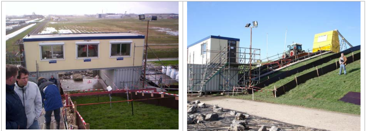
Figure 2-3: Impression of the test set-up with the measuring cabin on top the two containers
