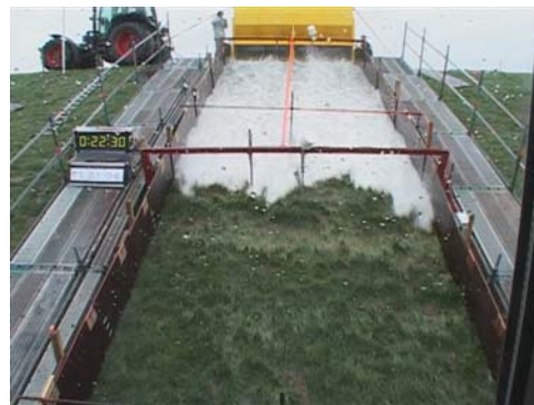
Figure 9-10: Situation during overtopping of 0,1 l/s/m. The biggest wave shown here had a volume of 0.7 m 3 per m width
