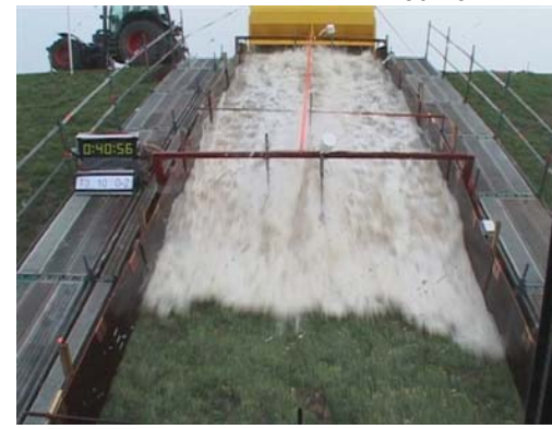
Figure 9-12: Situation during overtopping of 10 l/s/m. The biggest wave shown here had a volume of 2.5 m 3 per m width
