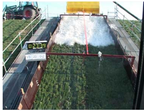
Figure 10-8: Situation during overtopping of 20 l/s/m. The biggest wave shown here had a volume of 3.5 m 3 per m width
