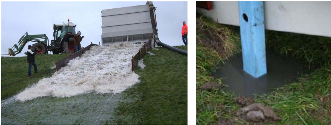
Figure 4-5: Trial testing of the wave overtopping simulator (left) and penetration of footing in subsoil (right)
