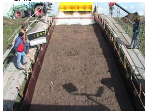
Figure 11-8: Situation during overtopping of 1 l/s/m. The biggest wave shown here had a volume of 1 m 3 per m width
