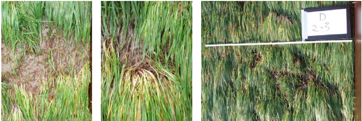
Figure 9-1: Detailed photographs of some bare spots after the 1 l/s/m test at the unreinforced test section
