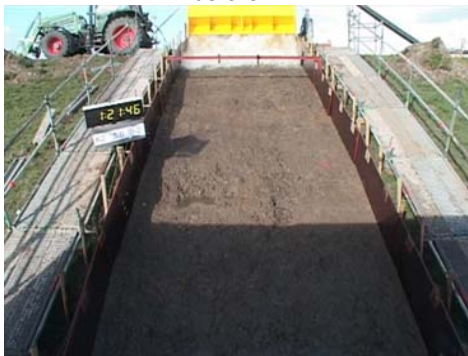
Figure 11-9: Situation during overtopping of 5 l/s/m. The biggest wave shown here had a volume of 2.0 m 3 per m width
