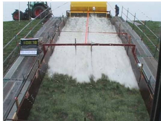
Figure 9-11: Situation during overtopping of 1 l/s/m. The biggest wave shown here had a volume of 1 m 3 per m width
