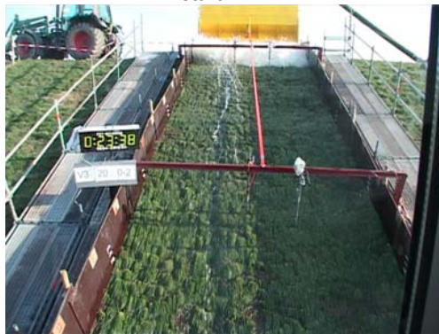
Figure 10-8: Situation during overtopping of 20 l/s/m. The biggest wave shown here had a volume of 3.5 m 3 per m width
