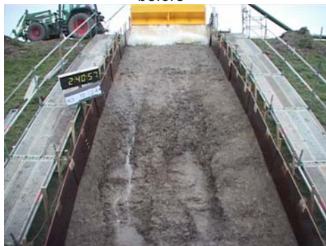
Figure 11-10: Situation during overtopping of 10 l/s/m. The biggest wave shown here had a volume of 2.5 m 3 per m width
