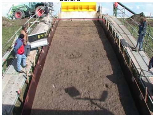
Figure 11-8: Situation during overtopping of 1 l/s/m. The biggest wave shown here had a volume of 1 m 3 per m width
