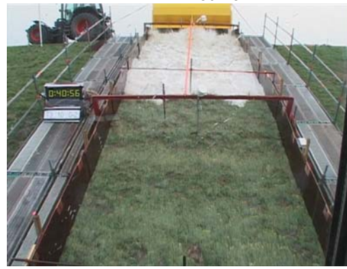
Figure 9-12: Situation during overtopping of 10 l/s/m. The biggest wave shown here had a volume of 2.5 m 3 per m width
