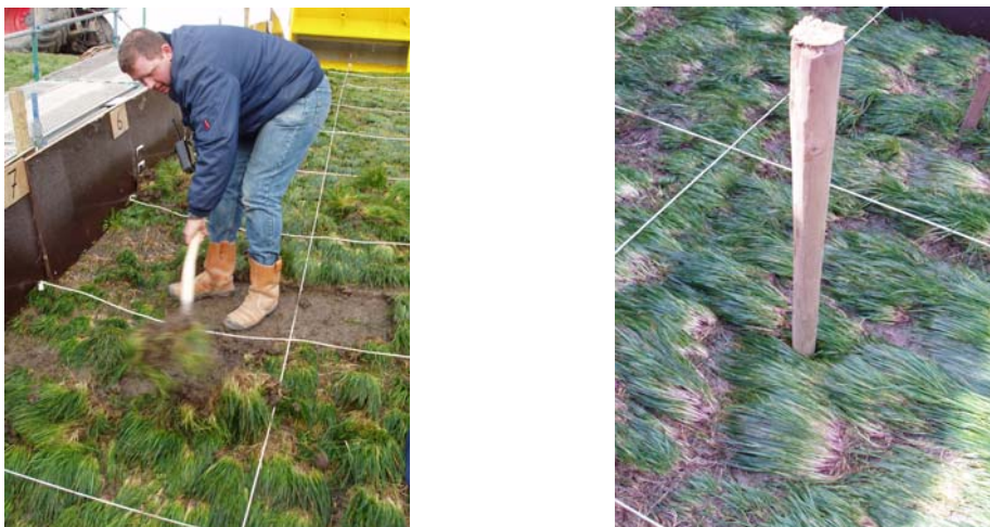
Figure 2-6: Introducing damage; removal of the upper grass layer with horizontal dimensions 1*1 m and placing a pole with a diameter of 0.07 m.
