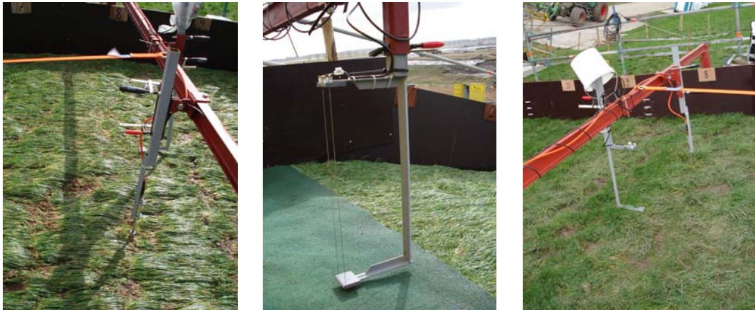
Figure 7-1: 1) velocity meter (EMS), 2) wave thickness meter (GHM) and 3) both meters fixed to a measuring frame
