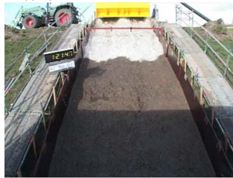
Figure 11-9: Situation during overtopping of 5 l/s/m. The biggest wave shown here had a volume of 2.0 m 3 per m width
