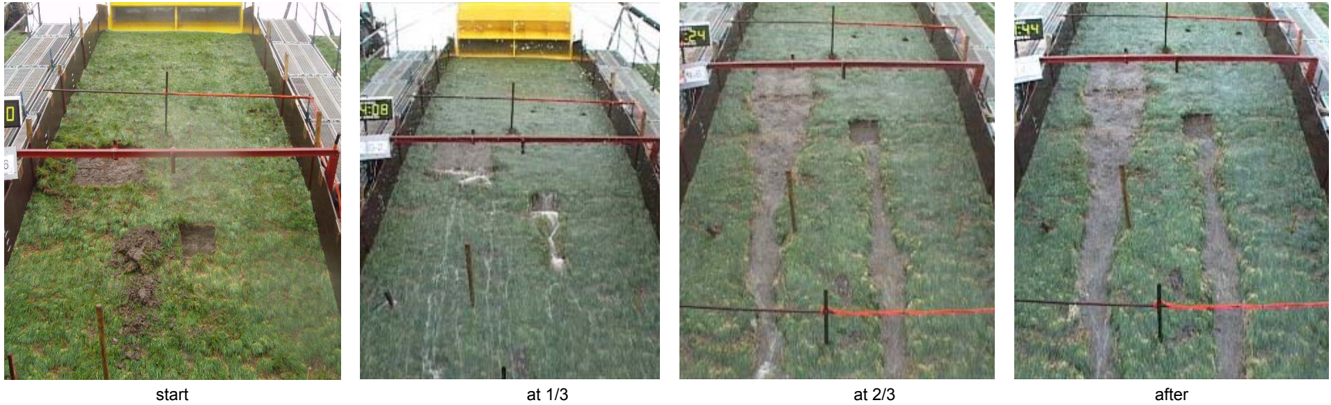
Figure 9-16: Situation during overtopping of '50' l/s/m with initial damage. The biggest wave had a volume of 3.5 \text{ m}^3 per m width (see Figure 9-10)
