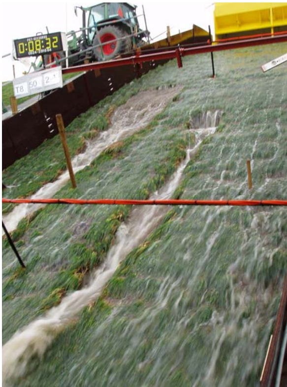
Figure 9-9: Typical flow concentration at the gullies
