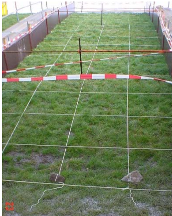
Figure 6-2a: Location of the water tension meters (poles)
