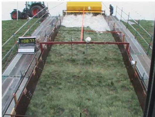
Figure 9-11: Situation during overtopping of 1 l/s/m. The biggest wave shown here had a volume of 1 m 3 per m width
