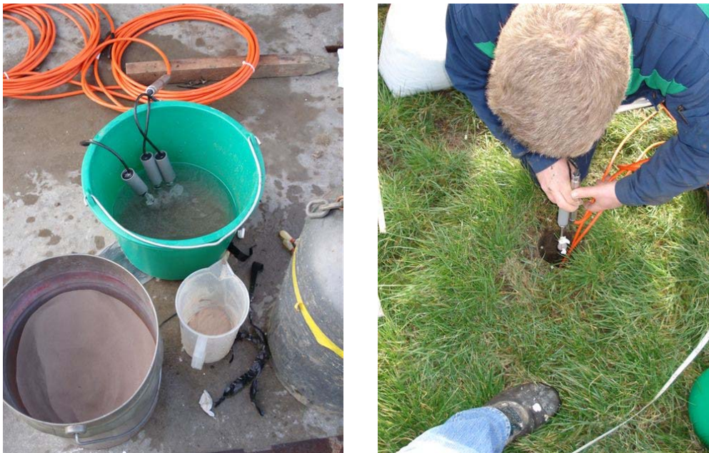
Figure 6-1: Preparations and placing of the water tension meters at the unreinforced test section
