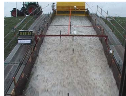
Figure 9-10: Situation during overtopping of 0,1 l/s/m. The biggest wave shown here had a volume of 0.7 m 3 per m width
