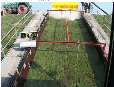
Figure 10-7: Situation during overtopping of 10 l/s/m. The biggest wave shown here had a volume of 2.5 m 3 per m width
