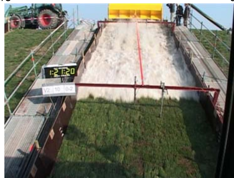
Figure 10-7: Situation during overtopping of 10 l/s/m. The biggest wave shown here had a volume of 2.5 m 3 per m width
