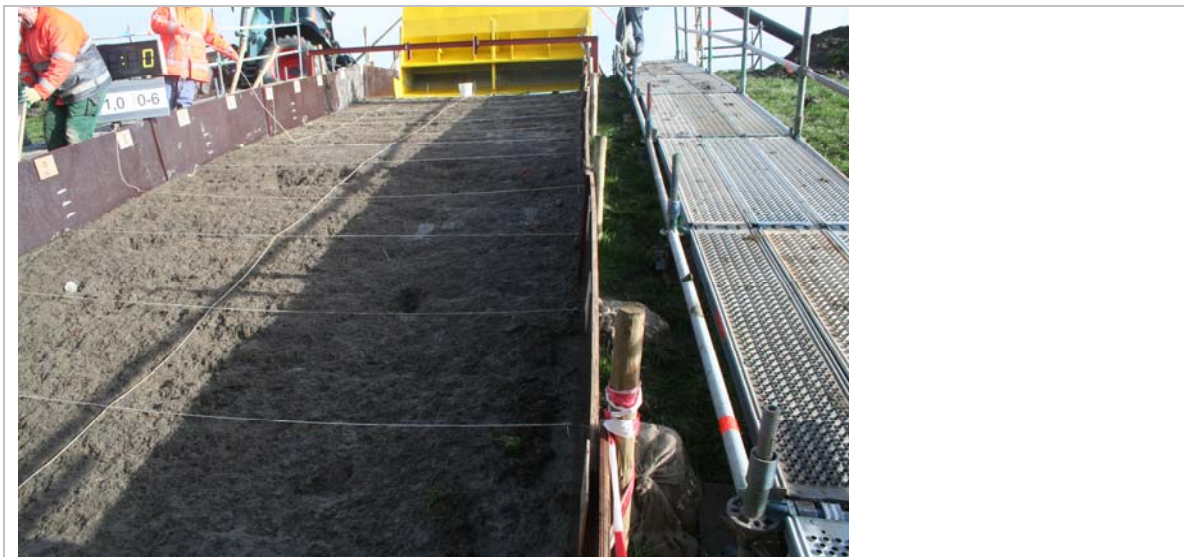
Figure 11-2: Impression of starting erosion of bare clay surface after interrupted 0.1 l/s/m test
