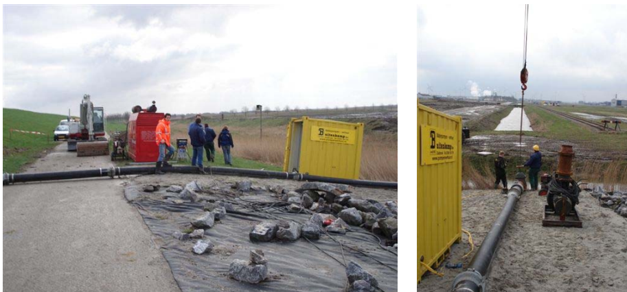
Figure 2-5: Impression of pumping system: control room (yellow box), power supply (red trailer) and hose system towards the simulator
