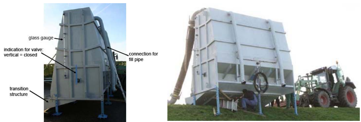
Figure 4-4: Side view of the simulator (left) and rear view (after placement for trial testing at the dyke)
