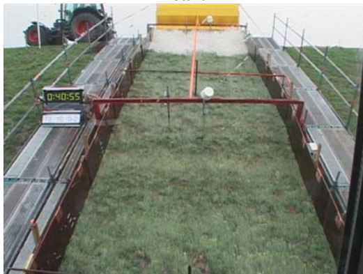
Figure 9-12: Situation during overtopping of 10 l/s/m. The biggest wave shown here had a volume of 2.5 m 3 per m width
