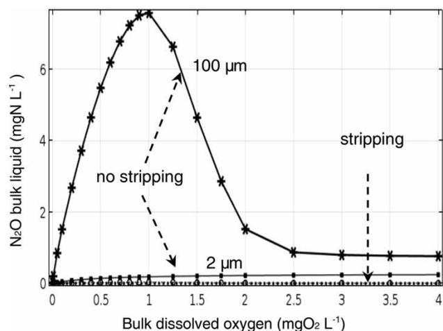
**Figure 3** | N<sub>2</sub>O bulk liquid concentration for nitrifying conditions as a function of bulk O<sub>2</sub> for a 2 μm suspended growth and 100 μm biofilm system, with stripping (solid line) and without stripping (dashed line).
