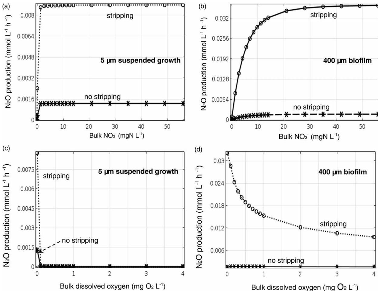
**Figure 5** | N<sub>2</sub>O production rates in denitrifying biofilms with a constant biofilm surface area, with and without stripping, for a 5-μm biofilm (‘suspended growth’) (a), (c) and 400-μm biofilm (b), (d) as a function of bulk NO<sub>3</sub><sup>-</sup> (a), (b) and (c), (d) as a function of bulk O<sub>2</sub>.
