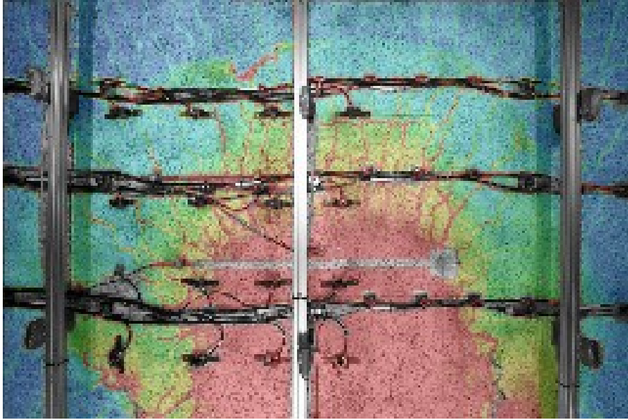
Figure 7.9: DIC image of flexure induced punching failure of SR1M1
