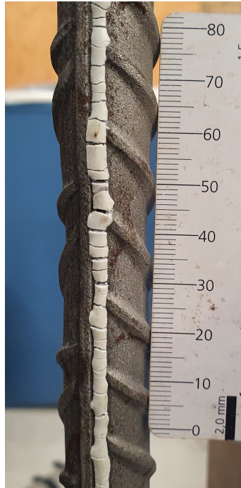
Figure 6.8: Cracks in the glue after yielding
