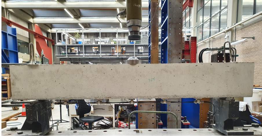
Figure 6.9: Setup of the small beam tests
