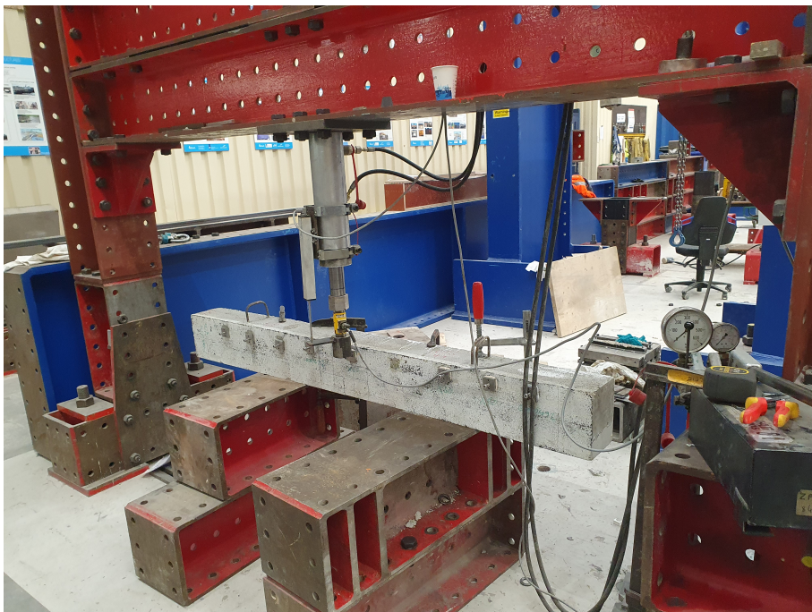
(b) Loading by manual hydraulic jack
