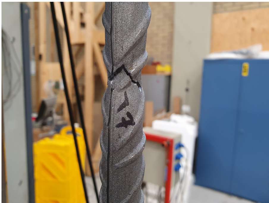
Figure B.19: failure T7
