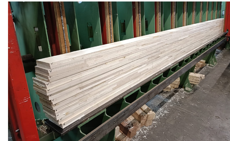
Figure 3: Fingerjointed and laminated poplar beams
