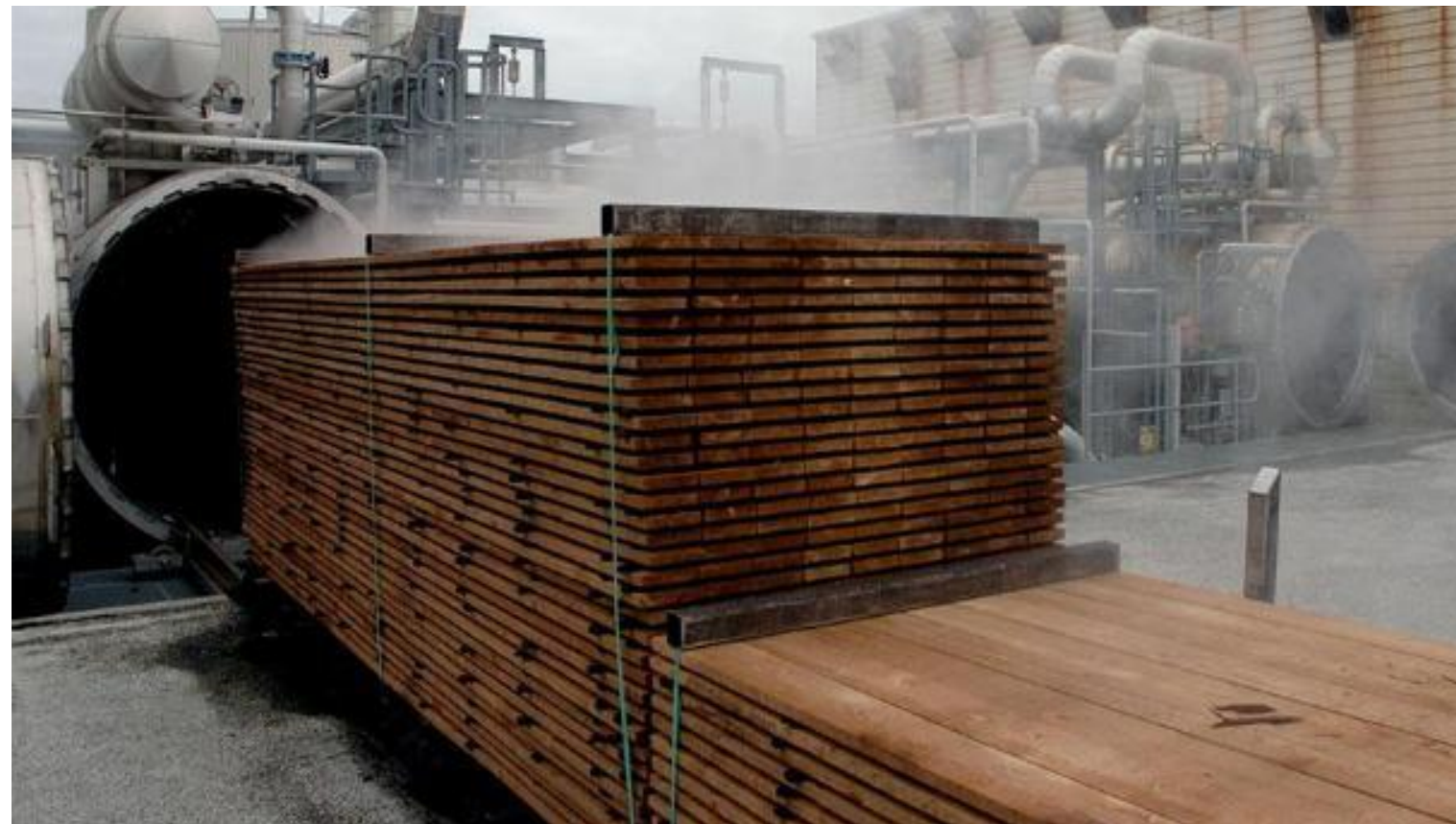
Figure 1: Thermal modification - PLATO
