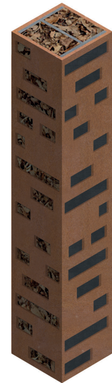
Figure 112.3. Corten steel pillar.
