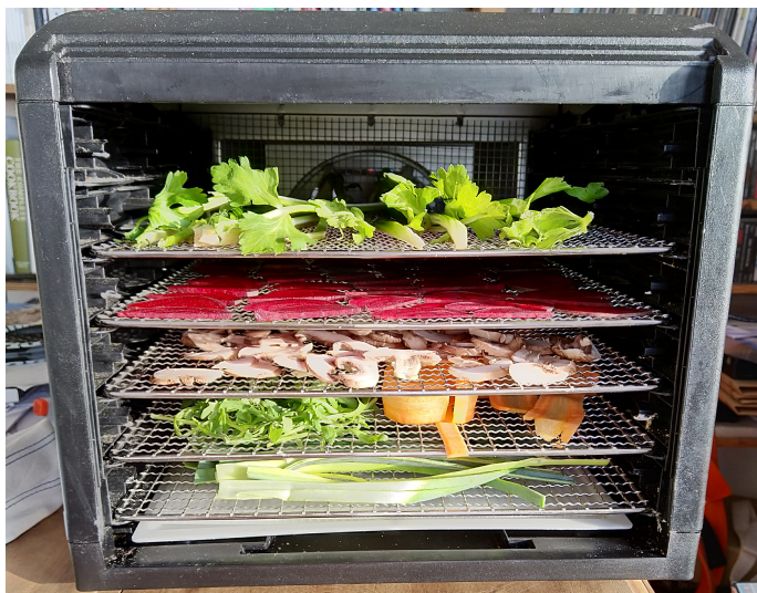
Figure 25 Professional dehydrator used to make the testing powders. Due to its size, large batches could be made quickly.
