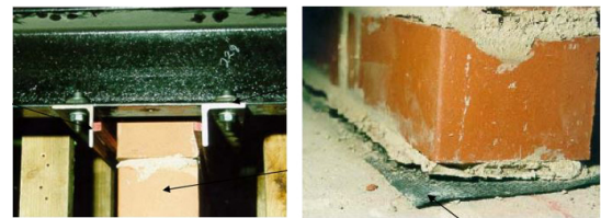
Figure 3.3: Details of supports experiment Doherty (left: top support, right: bottom support) [Doherty, 2000]
