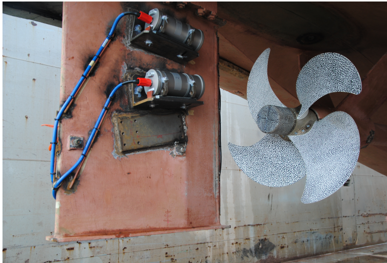
Figure 6: Starboard rudder side with cameras.
