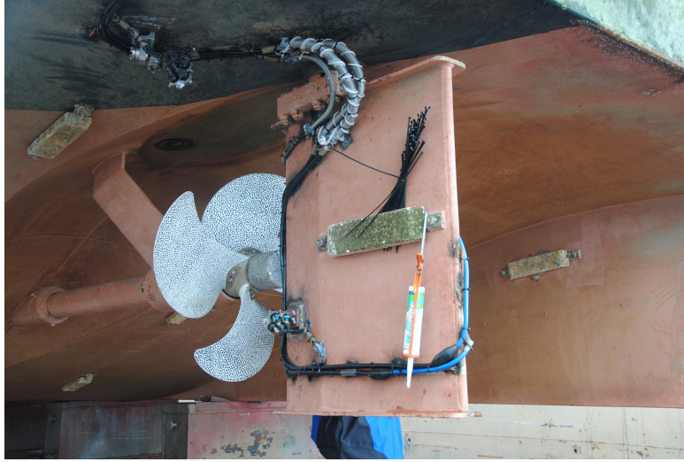
Figure 7: Lights on rudder and hull and cables.
