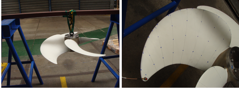
Figure 5: Images taken during the natural frequency measurements of the composite blades.
