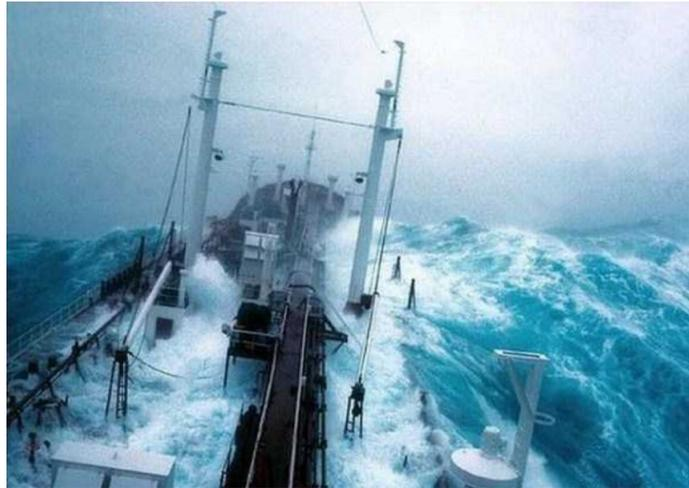
Figure 1.1: Green water on a ship offshore (Source:www.restnova.com)
