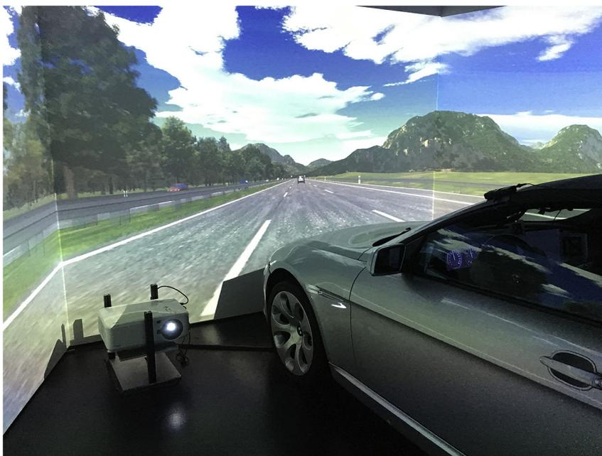
Fig. 1. Driving simulator used in the experiment.
