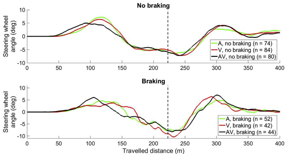
**Fig. 4.** Mean steering wheel angle across all take-overs for take-overs in which the driver braked (bottom) or did not brake (top). If the participant overtook the car on the right, the sign of the steering wheel angle was reversed. The dotted black line represents the location of the stationary vehicle. A = Auditory, V = Vibrotactile, AV = Auditory & Vibrotactile.
