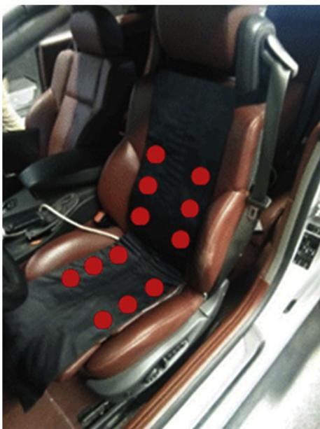
**Fig. 2.** Vibration mat on the driver seat of the simulator. Red circles indicate the approximate locations of the vibration motors. (For interpretation of the references to colour in this figure legend, the reader is referred to the web version of this article.)
