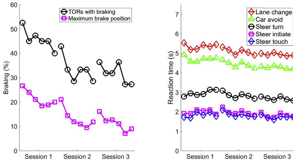
**Fig. 6.** Left: Percentage of take-over requests (TORs) that involved braking and mean maximum brake position across TORs as a function of the TOR number (3 sessions \* 6 TORs per session equals 18 TORs per participant). Right: Mean lane change times, mean car avoid times, mean steer turn times, mean steer initiate times, and mean steer touch times as a function of the TOR number. Markers of the six TORs within the same session are connected by a line.
