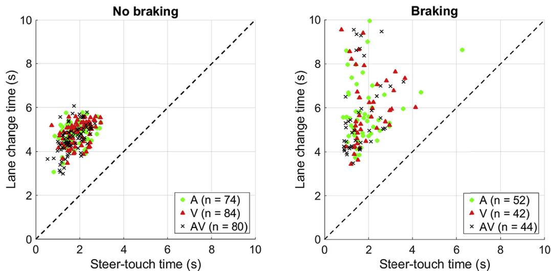
**Fig. 5.** Scatter plot of lane change time versus steer-touch time, distinguishing between trials in which the participant did not brake (left panel) and trials in which the participants braked (right panel). A = Auditory, V = Vibrotactile, AV = Auditory & Vibrotactile.
