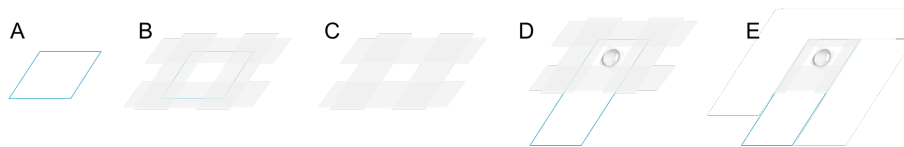
Figure 4.3: 1-3) peel the spin coated film of PPC from the cover slide using a rectangular window of Scotch tape. 4-5) attach the tape window to the glass slide such that the film covers the PDMS substrate.
