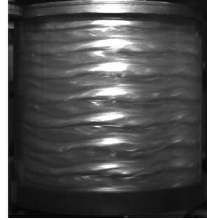
**Figure 3.16:** Snapshot of the TC cell with modulated waves at  $Re_i=1233$
