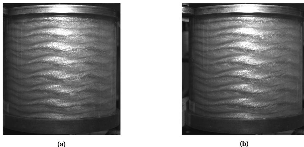
**Figure 4.18:** Snapshots of the TC system showing a reduction in number of azimuthal waves from 8 ( $Re_i = 811$ ) in (a) to 7 ( $Re_i = 866$ ) in (b) without a change in flow regime.
