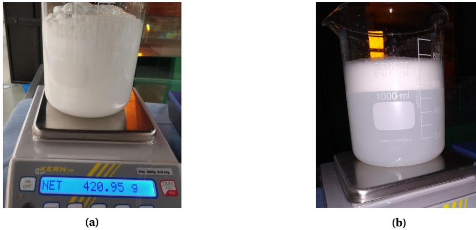
**Figure C.2:** (a) Gillette shaving foam weighed in the required proportion (b) Prepared solution with the top layer of foam to be removed.
