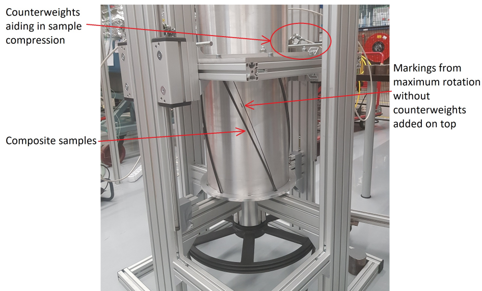
Figure 7.9: Room temperature (elastic) deformation of the composite samples
