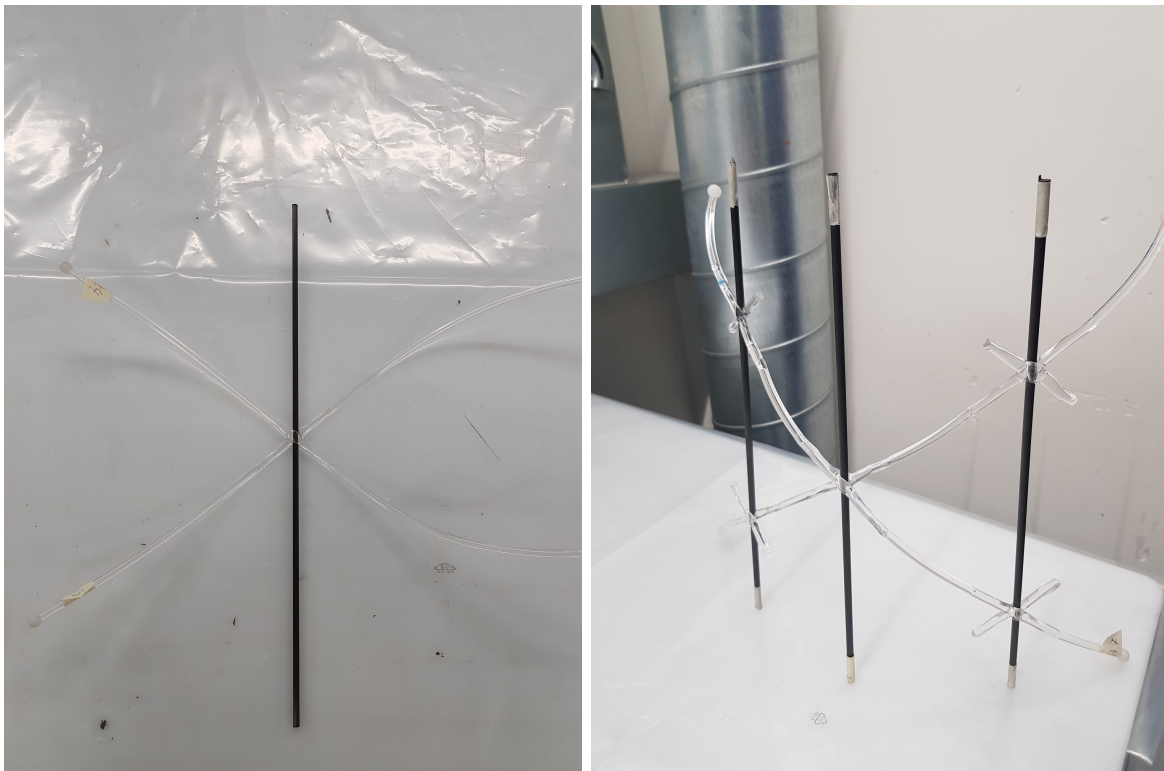
(a) Helical samples 4 and 5, welded to a single composite sample
