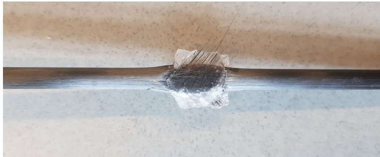
Figure 6.9: Close-up of the failure area in a shear test sample
