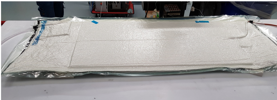
Figure 7.5: Vacuum bag containing aluminium plate with silicon heating blanket
