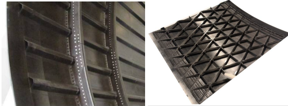
Figure 2.1: Difference between a conventional composite semi-monocoque structure (left [2]) and a grid stiffened structure (right [3])
