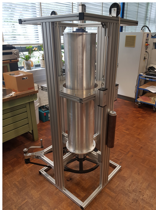
Figure 7.3: Completed setup of the Helical Winder Demonstrator, excluding heating method
