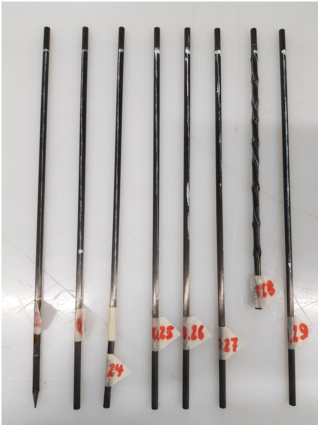
Figure A.2: Overview of the twisted samples O.22 to O.29
