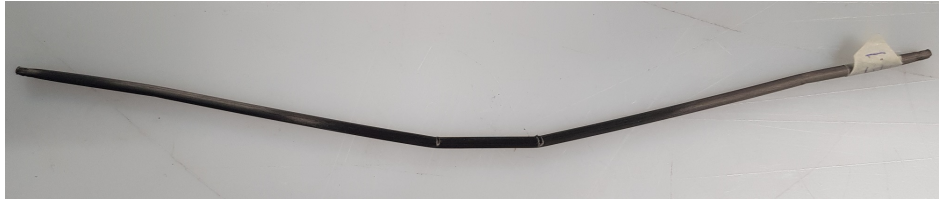
Figure A.4: Resistance heating sample after bending
