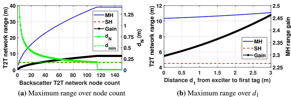
**Figure 5.3:** Maximum range of a one-dimensional T2T multi-hop network. Simulation parameters listed in Table 5.1. Node count is critical for range extension, while  $d_1$  hardly makes a difference. *SH*: single-hop, *MH*: multi-hop,  $d_N$ : inter-tag distance,  $d_{min}$ : minimum value of  $d_N$ .
