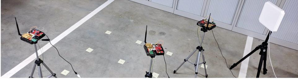
**Figure 6.2:** Photograph of the setup to evaluate phase cancellation countermeasures in T2T networks, discussed in Section 6.3: Three backscatter T2T tags on tripods, next to white panel antenna. Grid coordinates marked with yellow squares.
