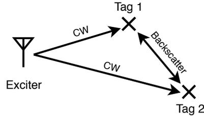
**Figure 3.2:** Backscatter T2T scenario. *CW*: continuous wave.
