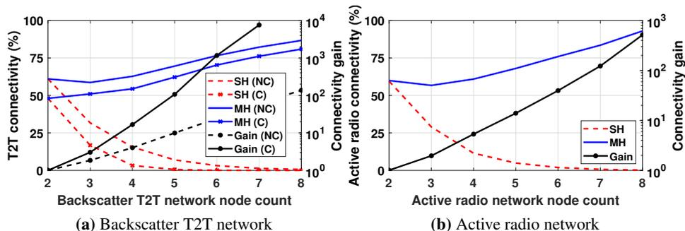
**Figure 5.2:** Numerical example of network connectivity with simulation parameters listed in Table 5.1. Fig. 5.2a: multi-hop versus single-hop full connectivity (*all* nodes connected with each other, either only directly, SH, or through other tags, MH) with and without phase cancellation; Fig. 5.2b: output power of tags ( $-6$  dBm) chosen to match connectivity of backscatter network; *SH*: single-hop, *MH*: multi-hop, *NC*: no phase cancellation, *C*: phase cancellation.
