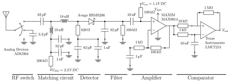
**Figure 3.4:** Backscatter T2T transceiver design with labeled logical blocks [5].
