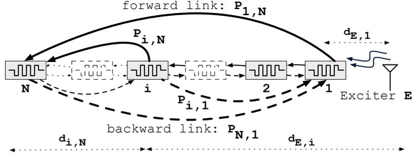
**Figure 4.2:** Diagram of multi-hop T2T received power analysis scenario.
