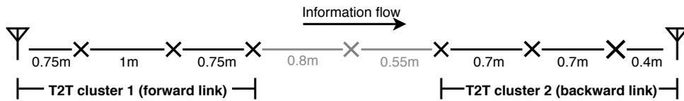
**Figure 6.4:** Two multi-hop T2T clusters are joined together by a bridging node.
