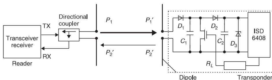
**Figure 3.1:** Working principle of a backscatter transponder [3].
