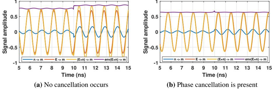
**Figure 4.1:** Normalized signals involved in T2T communication. From 5 to 10 ns, the source tag is backscattering a 0, and from 10 to 15 ns, a 1. The envelope of received signal varies according to backscattered symbol in Fig. 4.1a, but remains constant irrespectively in Fig. 4.1b.  $E$ : exciter,  $n$ : source tag,  $m$ : destination tag,  $env$ : envelope. Simulations according to parameters of Table 5.1.
