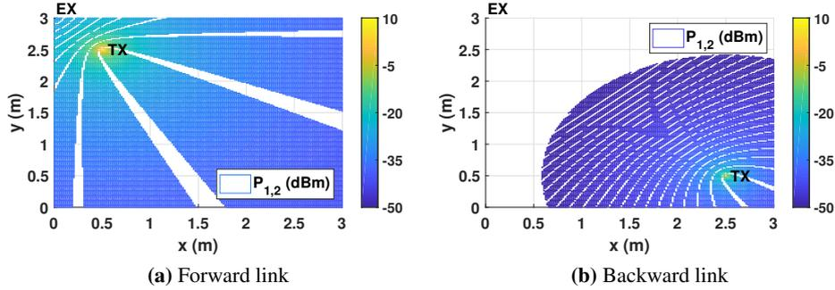
**Figure 5.1:** Pairwise tag connectivity with simulation parameters of Table 5.1. *EX* and *TX* mark the positions of the exciter and transmitter, respectively; receiver position variable. Phase cancellation bands are clearly visible. Fig. 5.1a transmitter can cover the network area. Fig. 5.1b transmitter offers limited coverage.
