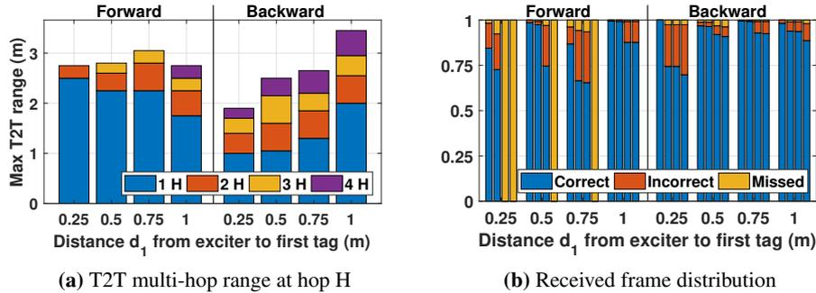
**Figure 6.1:** T2T link metrics for forward and backward link. Fig. 6.1a: the backward link has a higher multi-hop gain, *doubling the range* as receiving tag moves away from the exciter; Fig. 6.1b: frame distribution per hop (ordered from left to right in each bar group)—backward link is less prone to errors .
