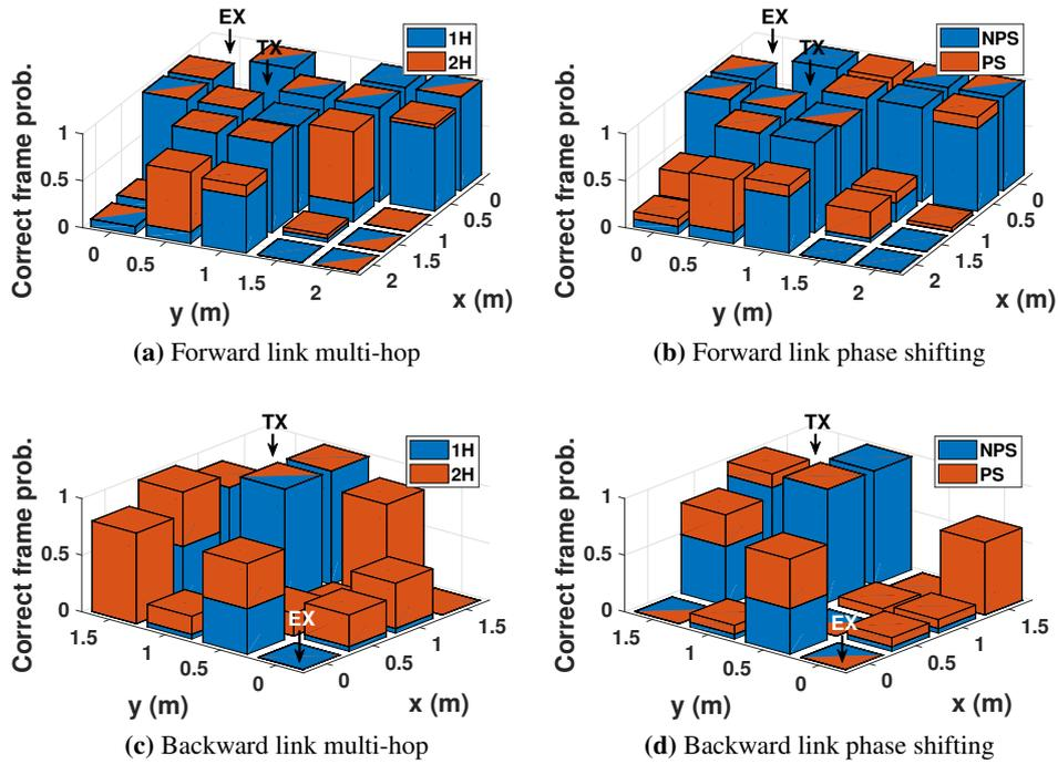
**Figure 6.3:** Backscatter T2T network phase cancellation experiment. *EX* and *TX* mark the positions of the exciter and transmitter, respectively. (*N*)*PS*: (no) phase shifting. Fig. 6.3a and 6.3b: forward link. Both methods yield comparable results. Fig. 6.3c and 6.3d: backward link. Multi-hop is superior in network coverage. Note: *1H* and *NPS* is the same case.
