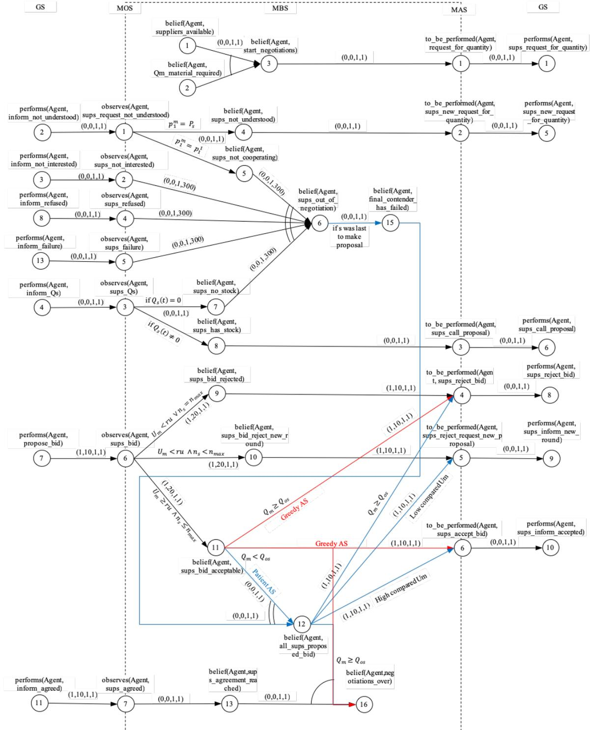
Figure 5.3: Graphical LEADSTO specification of manager for SC2
