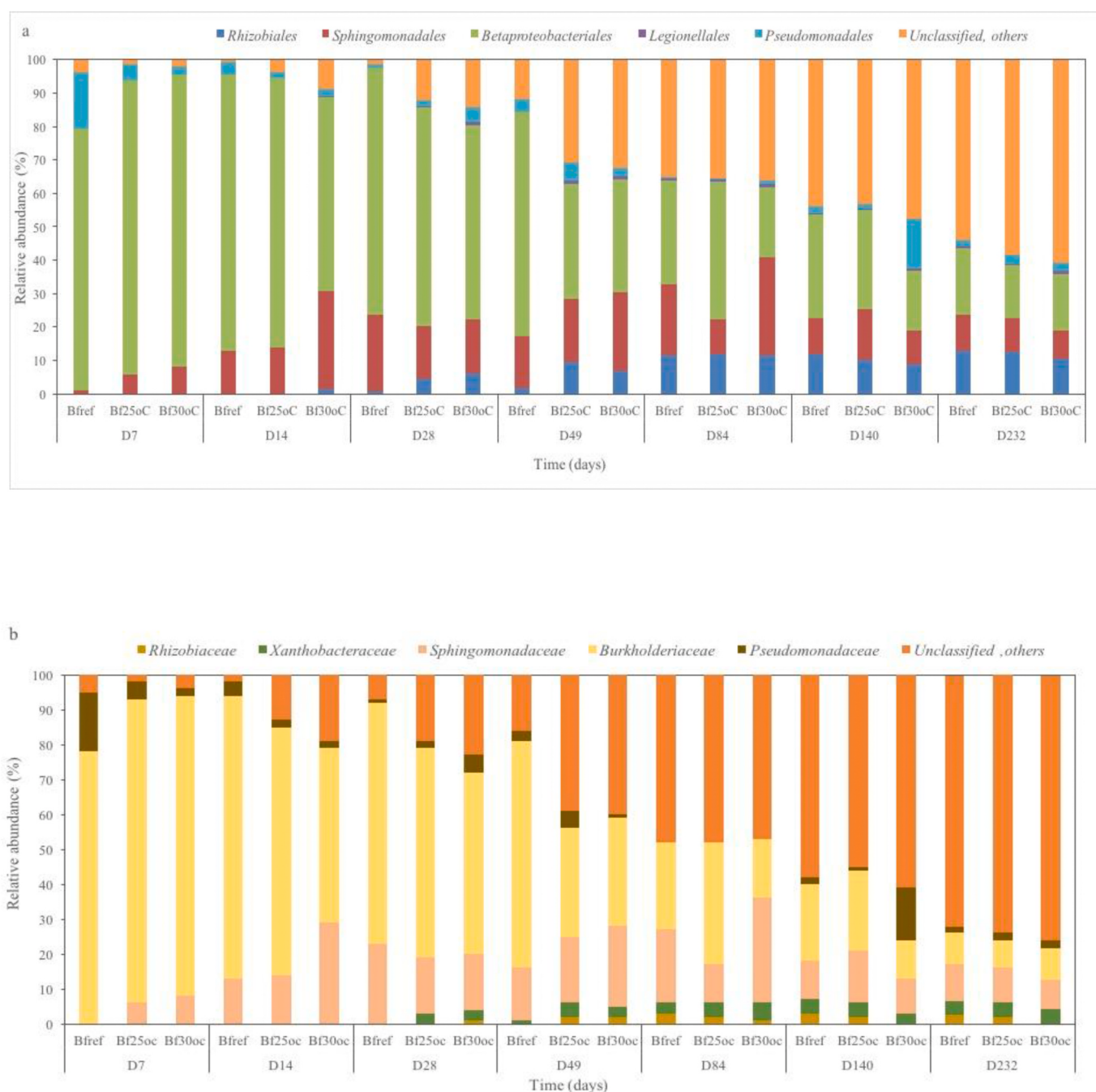
Fig. 4. Microbiome of biofilms shown as relative abundances (%) of core microbial groups, at both Order (a) and Family (b) level of taxonomic classification, from three sampling locations, developed within pilot distribution systems (Bf ref = biofilm from reference system, Bf 25°C = biofilm formed after cold recovery ( T_{max} = 25 °C), Bf 30°C = biofilm formed after cold recovery ( T_{max} = 30 °C)).
