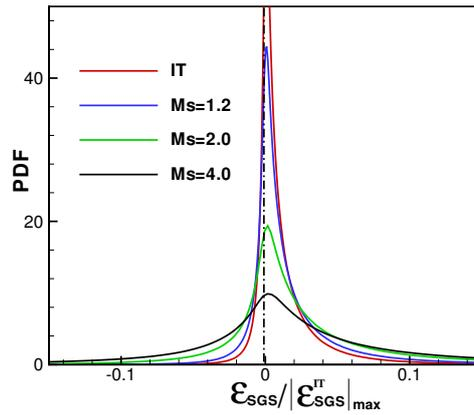
**Figure 1.** PDF of SGS dissipation for IT and post-shock turbulence at several shock Mach numbers. Negative values are associated with backscatter. The IT PDF data corresponds to the whole 3-D domain, while post-shock data corresponds to the plane of maximum amplification of the streamwise Reynolds stress.
