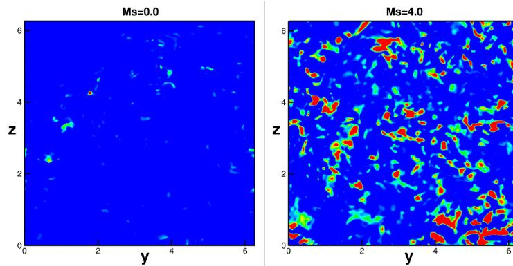
**Figure 2.** Distribution and magnitude of backscatter (negative values of SGS dissipation) in a) IT and b) in the transverse plane corresponding to the maximum amplification of the streamwise Reynolds stress after a  $M_s = 4$  shock.
