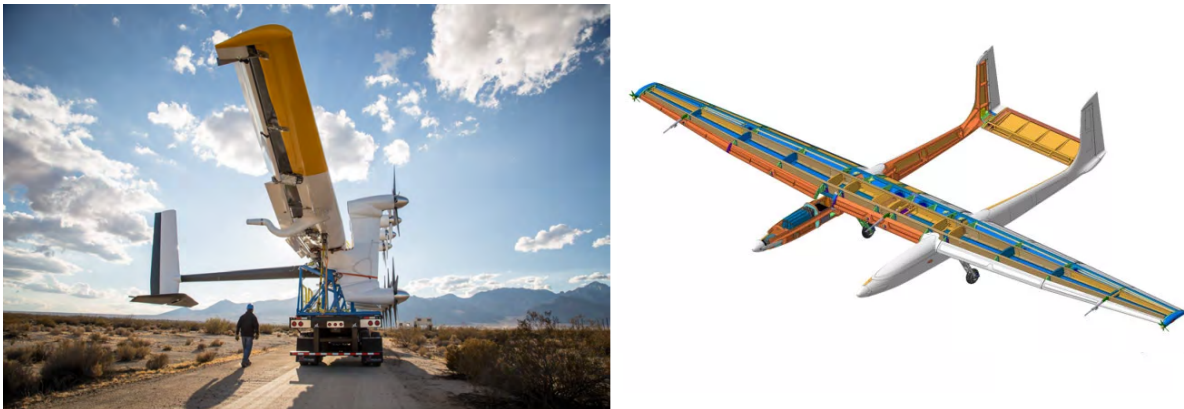
Figure 2.1: Examples of rigid monoplanes applied to AWE systems: M600 [13] (left) and AP-3 [14] (right)
