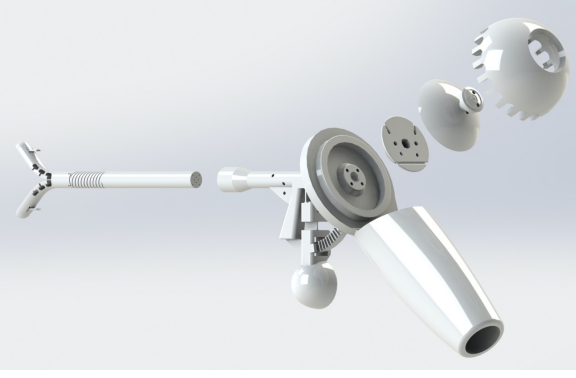
Figure 42: Exploded view of a 3D drawing of the LapaJoy containing 5 parts in total.
