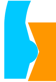
Figure 32: Schematic drawing of dome connection to base. Blue: dome. Orange: connection base.
