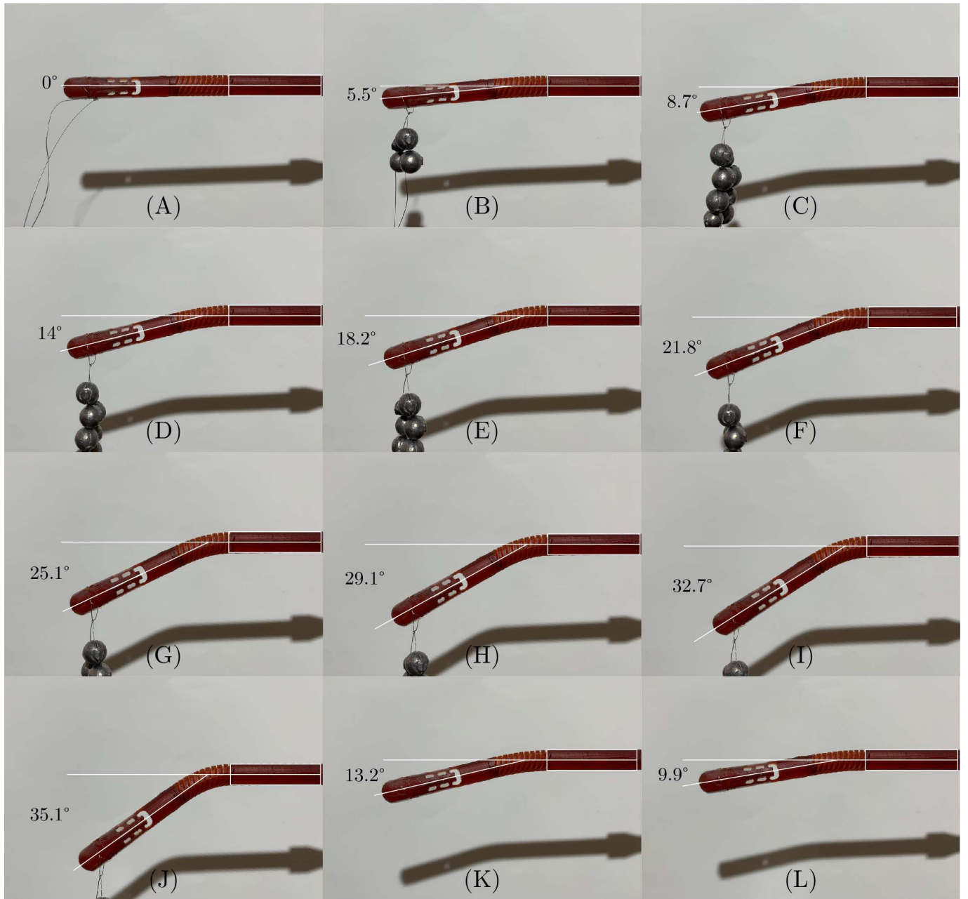
Figure 52: Bending force test by applying weights. A) Initial state. B-J) 10 grams of weight added for each step with the new bending angle. K) Directly after removing weights. L) After 25 minutes of removing the weights.
