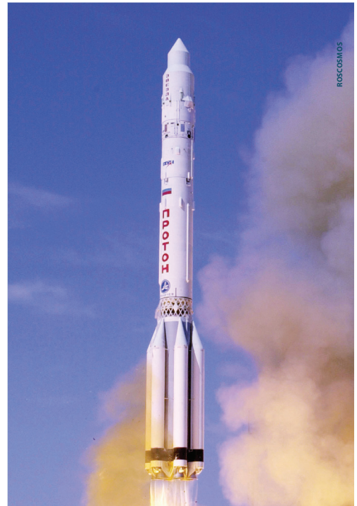
Figure 2. Proton Launch, toxic yellow fumes originating from the UDMH and NTO propellants
