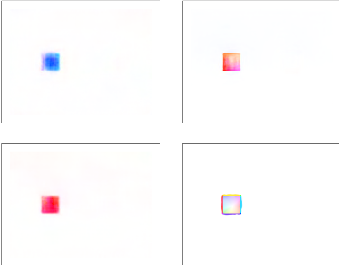
Figure 9.4: (all) Flow estimation produced by the four different models for \mathbf{v} = (218, 0) corresponding to a bright red ground truth color. Note that the color coding is similar to Baker et al., 2011 is used and can be found in Appendix B. (top left) Flow map corresponding to the FlowNet2S model. The model predicts that the square is moving outward (to the left) of the frame. (top right) Flow map corresponding to the SpyNet model. At larger velocities SpyNet has difficulty matching the squares at different timesteps and the estimate contains multiple colors corresponding to different velocity angles. (Bottom left) Flow map corresponding to the FlowNet2C model. Also FlowNet2C has trouble matching the complete patch at high velocities. At high velocities FlowNet2C does have the best performance. (Bottom right) Flow map corresponding to the LDOF model. This model produces a flow estimate corresponding to disappearing edges and appearing texture.
