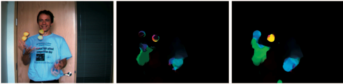
Figure 3.4: Illustration of large displacement of small structures. (left) The two input images overlaid. (middle) Flow field produced by Brox, Bruhn, Papenbergh and Weickert, 2004. The flow field color coding can be found in Appendix B with the exception that black instead of white corresponds to zero flow. (right) Flow field produced by Brox and Malik, 2011. Note the improved optical flow estimation for the hands and balls. Taken from Brox and Malik, 2011.
