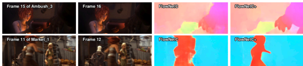
Figure 6.11: Flow predictions for different image pairs from MPI-Sintel. FlowNetC is retrained using training schedule with a disruptive learning rate. The retrained CNN is called FlowNetC+. Taken from Sun, Yang, Liu and Kautz, 2018.
