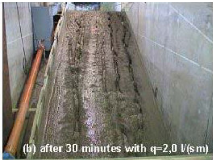
Photograph C.2: Pattern of clay erosion by wave overtopping
