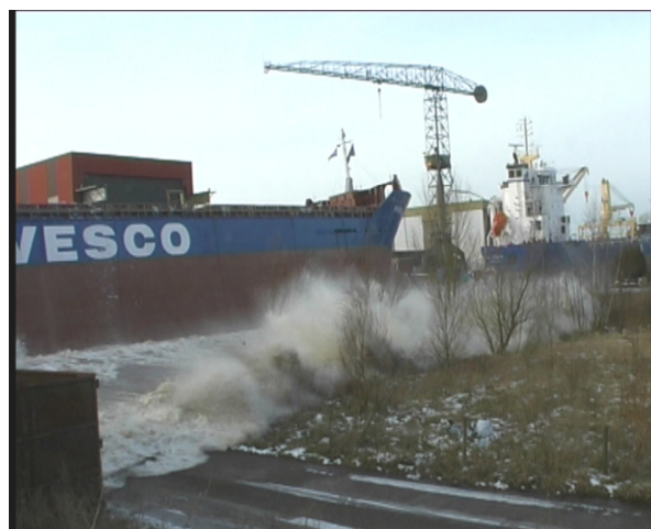
Figure 2.4: overtopping wave hitting vegetation
