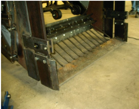
Figure 2.7: Cutting knife for uplifting of soil (courtesy Geerlings, Noordwijkerhout)
