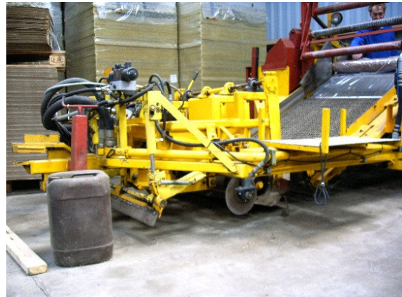
Figure 2.8: Conveyor belt for uplifting of soil (courtesy Queens Grass, Drouwen)
