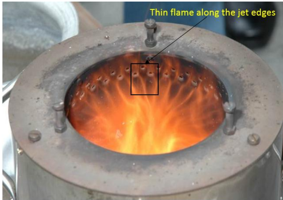
Figure 4.24: Flame pattern in the stove
