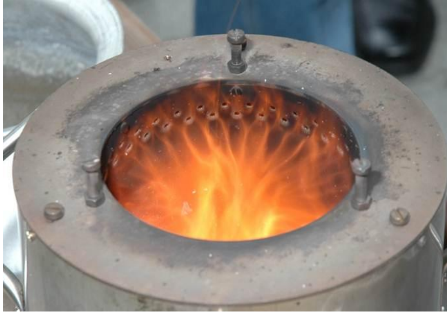
Figure 4.16: Flame pattern in the stove
