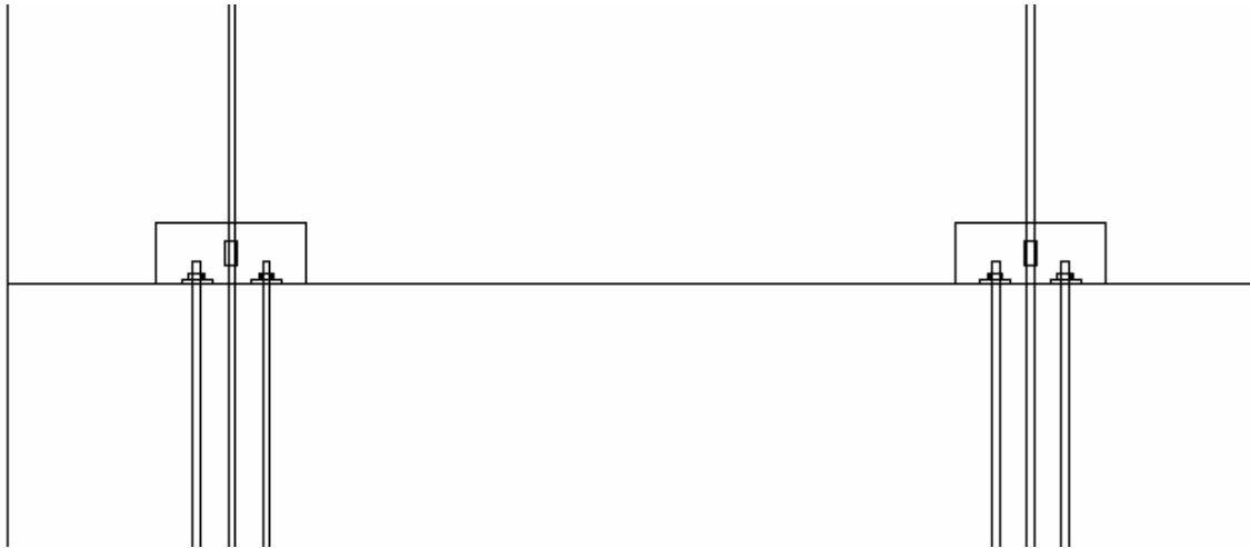
Figure 133: Principle of the proposed solution to anchor the core walls (indicative)
