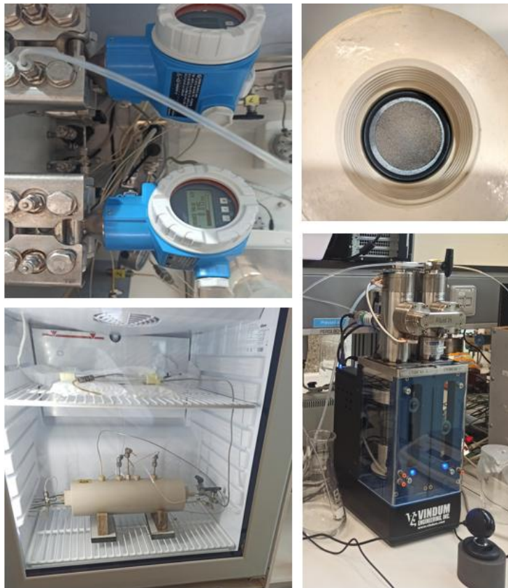
Figure 9: Pictures of the some of the parts that consist the fixed setup. On the top left are the differential pressure gauges (dP). Next to them is a picture of the core placed inside of the core holder. On the bottom left is a picture of the core holder placed inside the refrigerator. Lastly, on the bottom right there is a picture of the Vindum pump.
