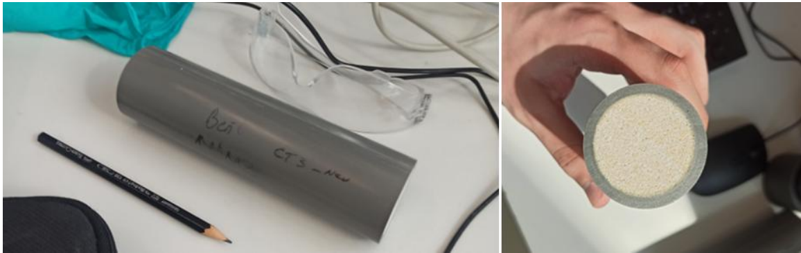
Figure 5: Pictures of a Bentheimer core sample that was used during the experimental work of this thesis. The core sample is surrounded by a grey colored glue.
