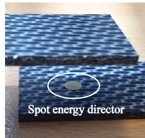
Figure 2.7: Spot energy director fixed on composite adherend prior to welding process.
