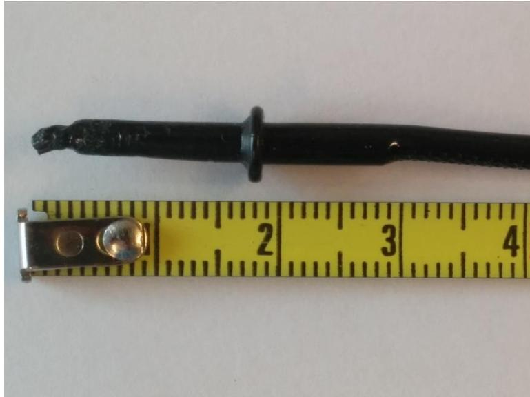
*Figure 43: Expanded section and ring of the second clog*
