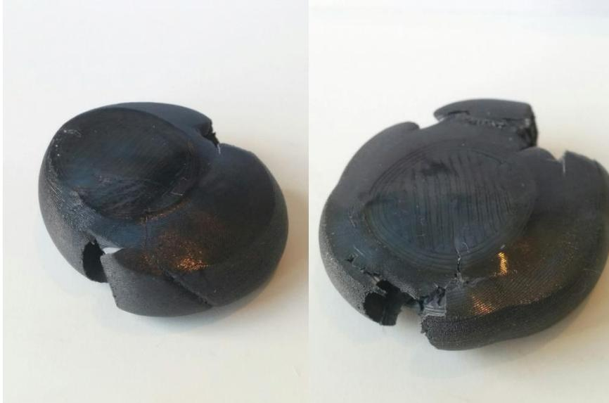
*Figure 79: MP-03-01-V and MP-03-10-A after compressive testing*
