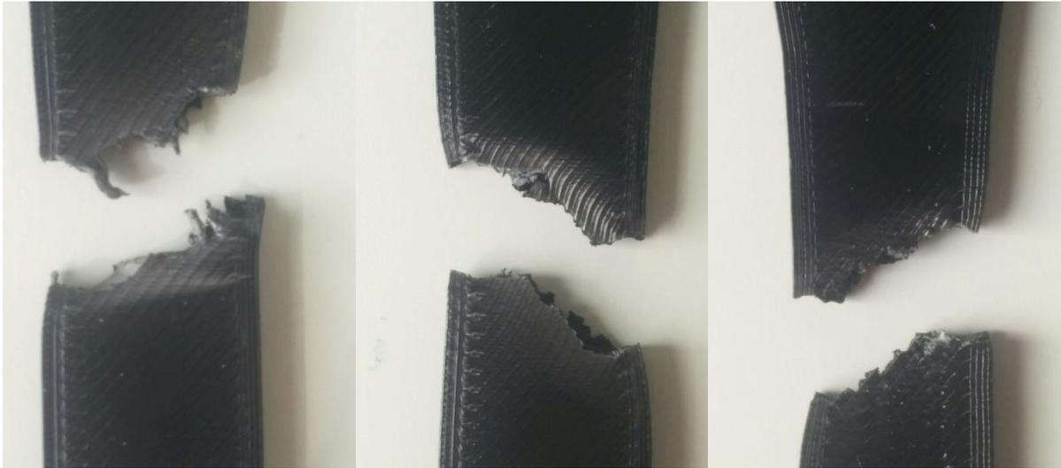
Figure 69: L-R, The fracture zones of MP-02-01-V (top), MP-02-03-V (top and bottom)
