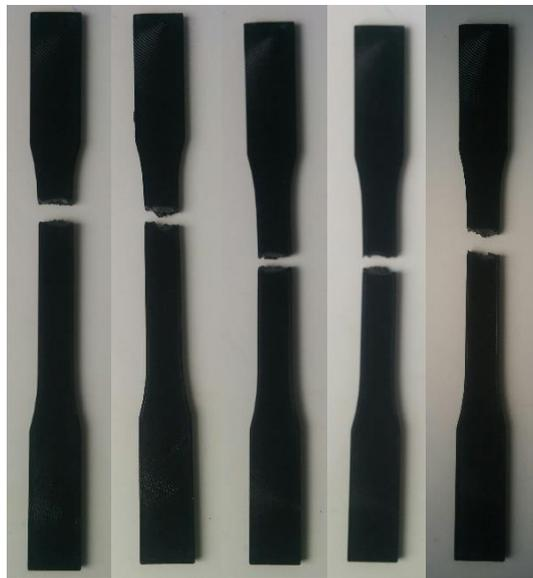
Figure 70: MP-02-06-A to MP-02-10-A (left to right) after testing
