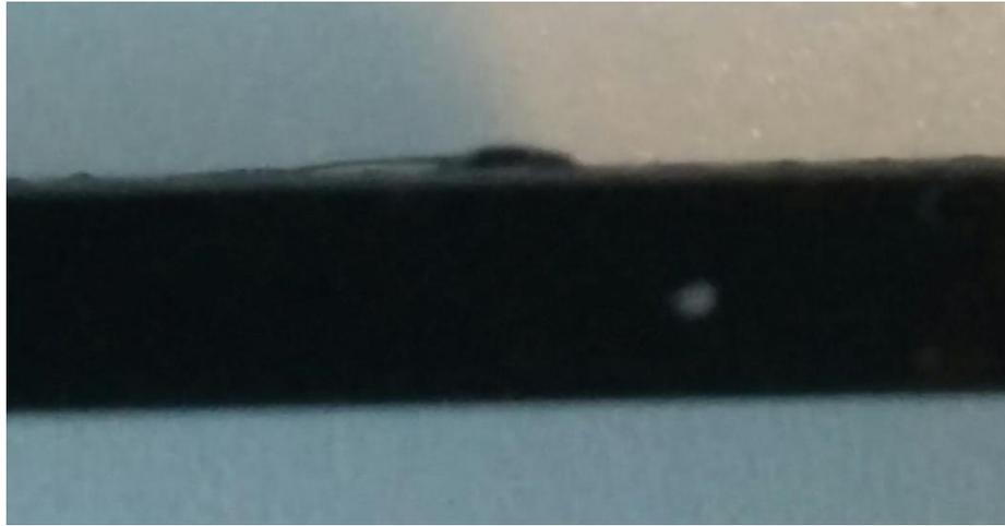
*Figure 54: Bulge on an MP-01 component*
