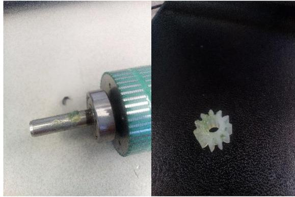
Figure 16: A servo motor (left) and a filament feed gear (right) showing green/grey lubricant
