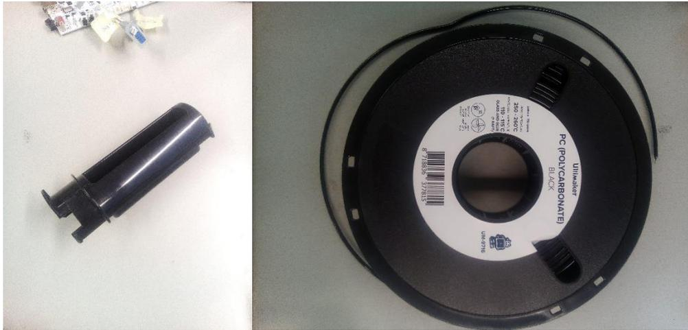
Figure 15: The filament spool holder (left) and the filament spool (right)
