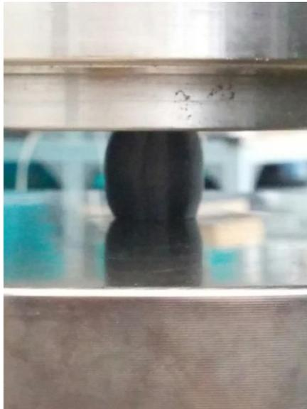
Figure 76: A MP-03 component deforming under high compressive load
