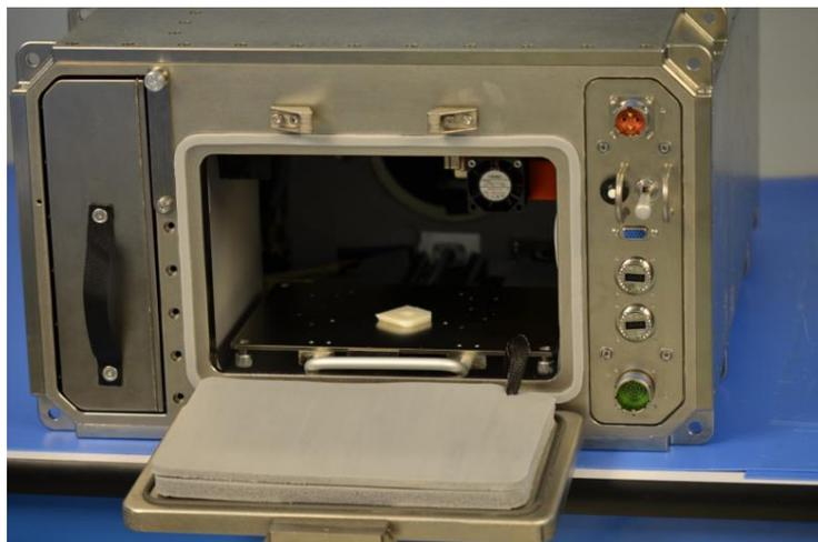
Figure 4: The AMF showing the print volume and a printed plastic component [11]
