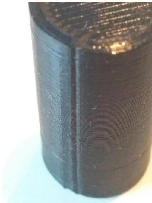
*Figure 58: The seam on an MP-03 component*
