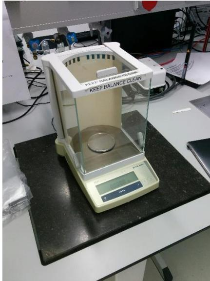
Figure 51: The Mettler Toledo Classic analytical balance used for mass analysis
