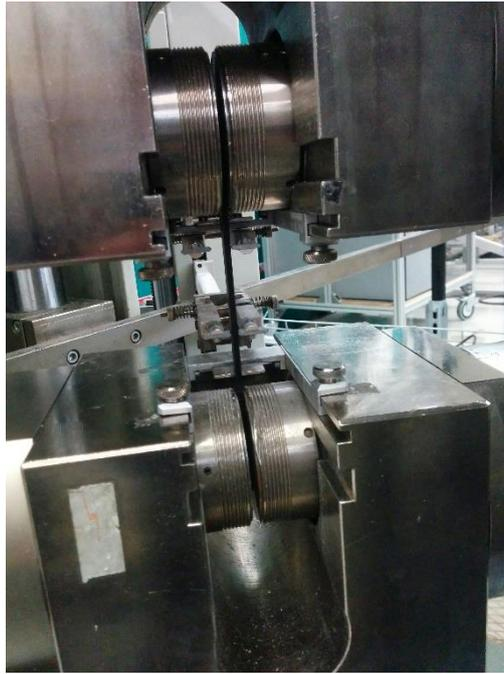
*Figure 65: Flexural testing set-up*
