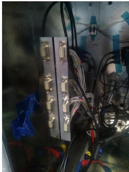
*Figure 18: The four Dsub connectors inside the vacuum chamber*
