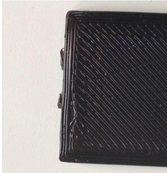
*Figure 57: Defect on bottom layer, end of MP-02 component*
