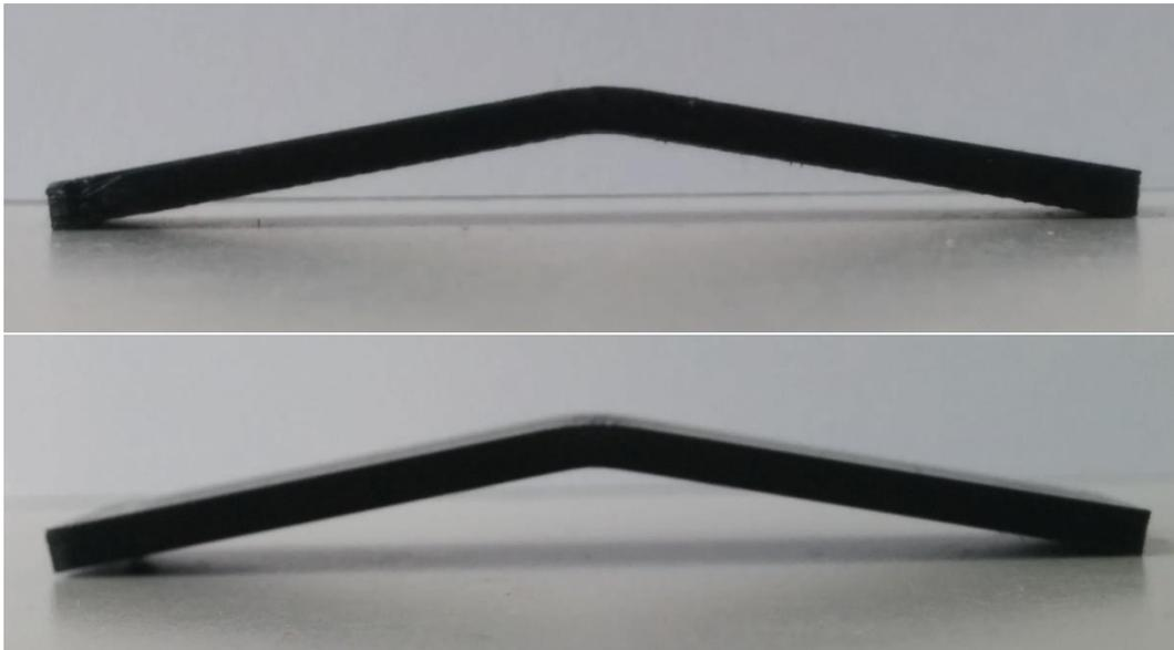
*Figure 62: MP-01-02-A and MP-01-07-V after flexural testing*
