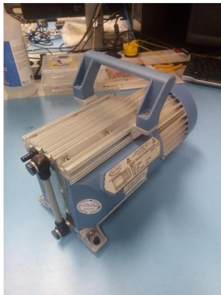
Figure 8: The vacuubrand MD-1 vacuum pump used for testing
