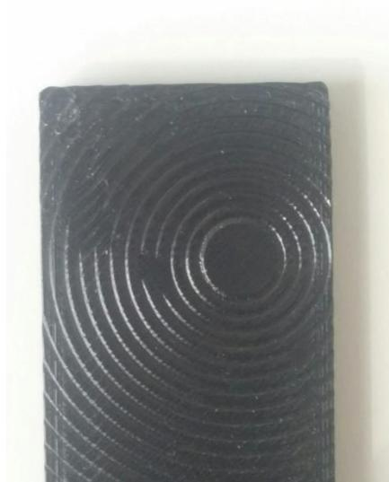
*Figure 72: The pattern of the pneumatic grips on MP-02-01-V*
