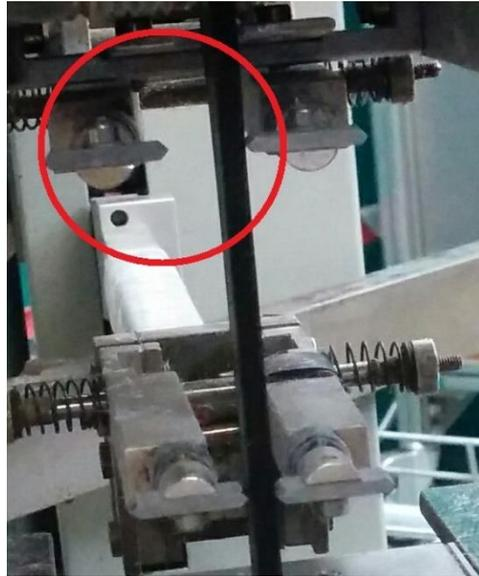
*Figure 66: Fouling of top extensometer grip*
