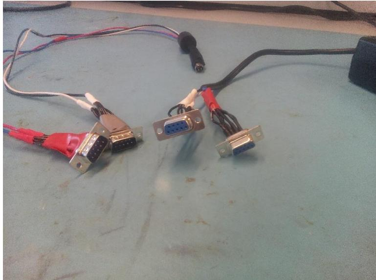
*Figure 19: the Dsub connectors on the rewired power supply*
