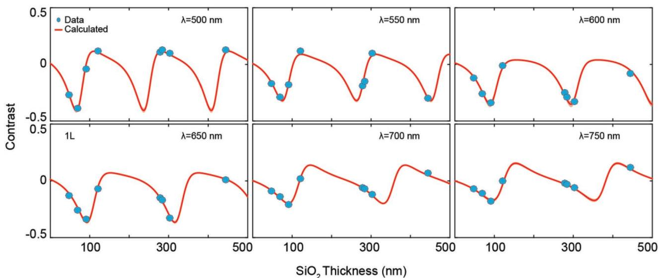
Figure 3. Optical contrast fitting of 1L  $\text{MoS}_2$  for different  $\text{SiO}_2$  thicknesses. The blue dots are the contrast data points for different thickness of  $\text{SiO}_2$  at specific wavelengths; the red lines are fits with the Fresnel equations, where the error of  $n$  and  $\kappa$  is minimized. The uncertainty of the calculated contrast is shown as the shaded regions, which is small and not visible in some cases.
