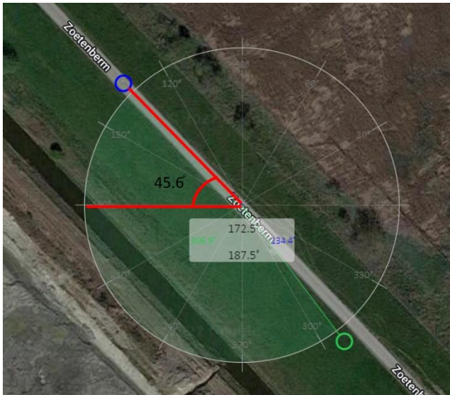
Figure 20: Angle between RD coordinate system and local coordinate system. Source: (Google Maps, 2022)
