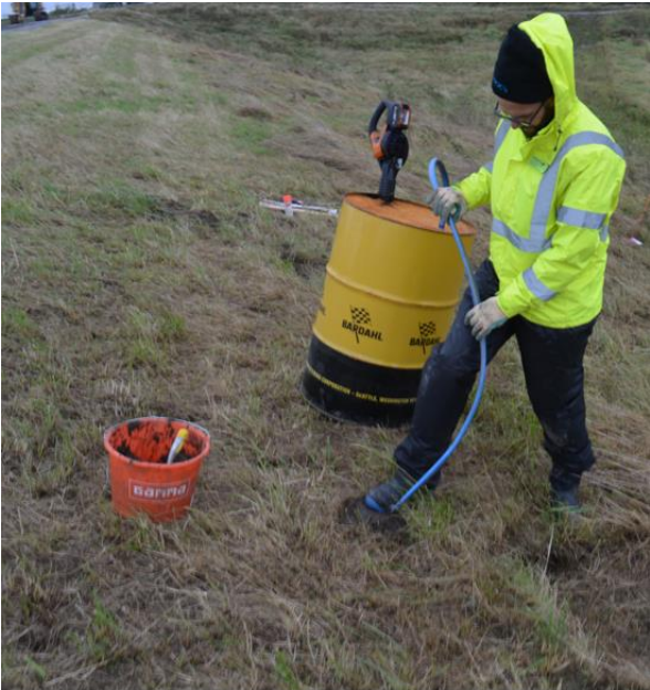
Figure 6: Smoke experiment procedure, using a leaf blower, smoke is blown from the barrel, through the rubber hose, into the burrow hole
