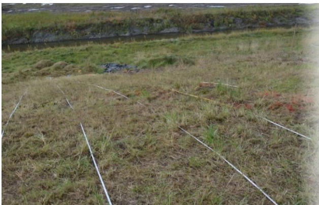
Figure 8: Coordinate grid used for GPR scans
