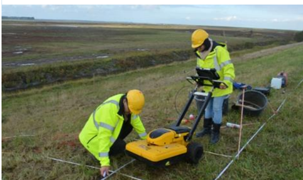
Figure 10: The GPR scanning a section of the levee
