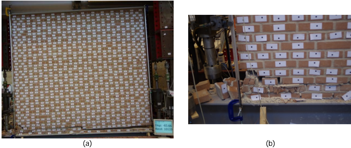
Figure 16 – Crack pattern of wall TUD_COMP-22 at the end of the test: (a) Overview; (b) Detail.
