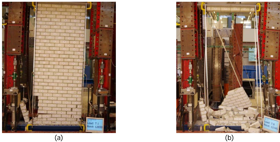
Figure 7 – Crack pattern of wall TUD_COMP-20: (a) Just before collapse; (c) At collapse.
