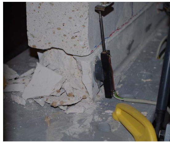
Figure 32 – Crack pattern of wall TUD_COMP-25 at the end of the test: (a) Overview; (b) Detail bottom-right corner.
