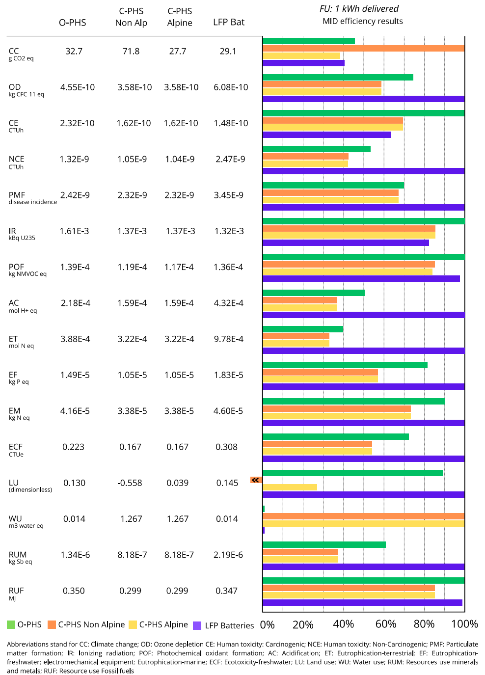
Fig. 7 Results for the 16 impact categories included in PEF. Negative results are depicted with a shortened bar rather than its value in maintaining graphic aesthetics
