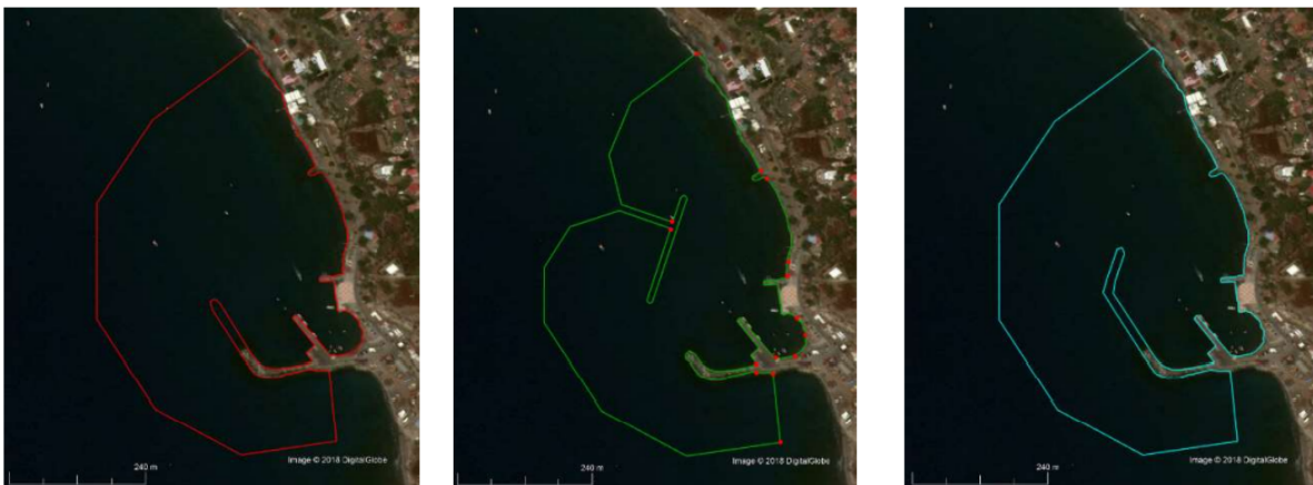
Figure 5.2: Three lay-out alternatives studied in detail by W+B (van der Leer et al., 2018).
