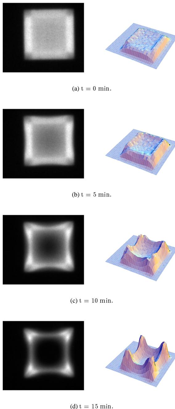
Figure 3: A series of images showing the evaporation process of ethyleneglycol-water (90%/10%,  $v/v$ ) in a vial at different times. Note that the images show the fluorescent intensity profile, *not* the shape of the meniscus.
