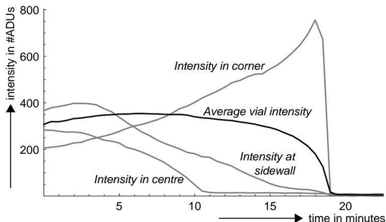
Figure 4: The average fluorescence signal from the vial, the signals from the center of the vial, the sidewalls of the vial and the corner of the vial as a function of time. It can be seen that, besides some geometrical effects, the average signal of the vial does not decrease during the evaporation process.
