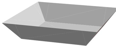
Figure 2: A  $200 \times 200 \times 20 \mu\text{m}^3$  wet etched square vial. The shape of the vial is a truncated pyramid.
