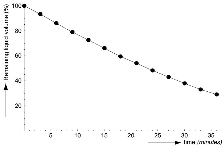
Figure 7: This figure shows the remaining liquid volume in the vial as a function of time. The evaporation speed is the slope of the line, which is almost constant, but decreases during evaporation.
