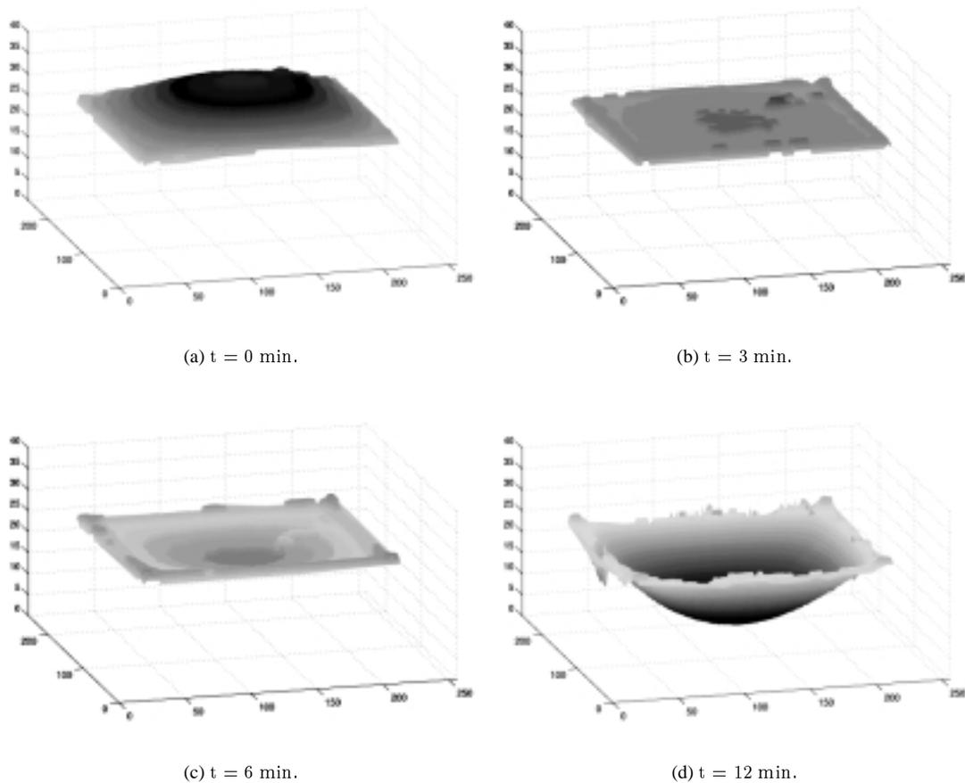
Figure 6: These figures show the shape of the meniscus of the liquid during evaporation. The edge of the meniscus connects to the border of the vial. The dimensions along the axis are voxel coordinates.
